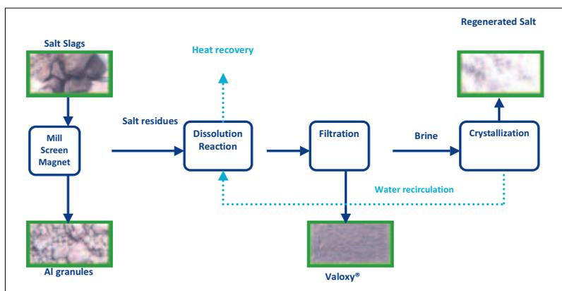
Fig. 5 RVA process flow chart showing three main outputs: aluminium granules, salt and Valoxy
