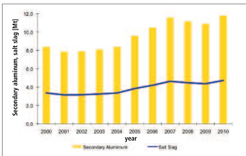
**Fig. 2** World arisings of salt slag – a function of secondary aluminium production
