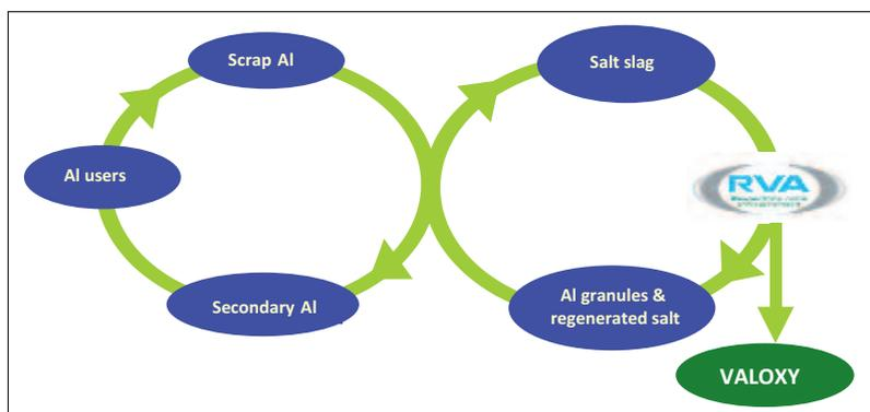
**Fig. 1** Material flows from salt slag to value-added raw materials
