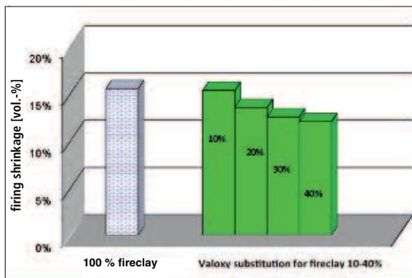
**Fig. 12** Volume firing shrinkage at 1250 °C resulting from partial substitution of fireclay by Valoxy®
