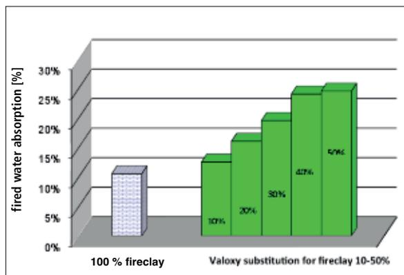
**Fig. 13** Fired water absorption at 1250 °C resulting from partial substitution of fireclay by Valoxy®
