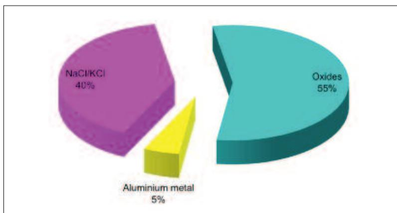
**Fig. 3** Typical composition of salt slag
