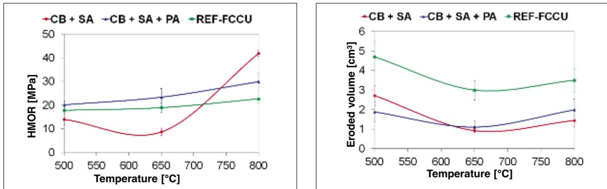
**Fig. 1** Hot modulus of rupture (HMOR) and eroded volume as a function of typical petrochemical temperatures (500–800 °C) for the designed compositions (CB+SA or CB+SA+PA) and for a commercial reference (REF-FCCU)
