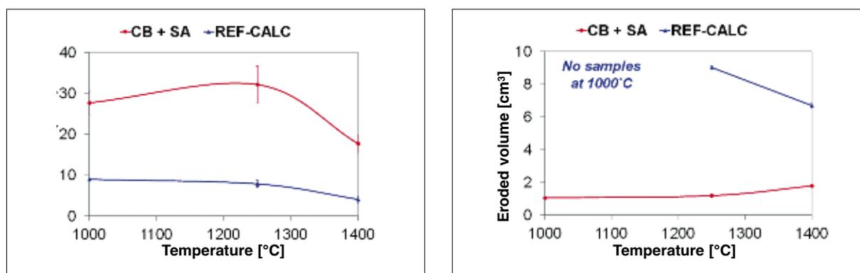
**Fig. 2** Hot modulus of rupture (HMOR) and eroded volume as a function of typical alumina calciner temperatures (1000–1400 °C) for the designed composition (CB+SA) and for a commercial reference (REF-CALC)
