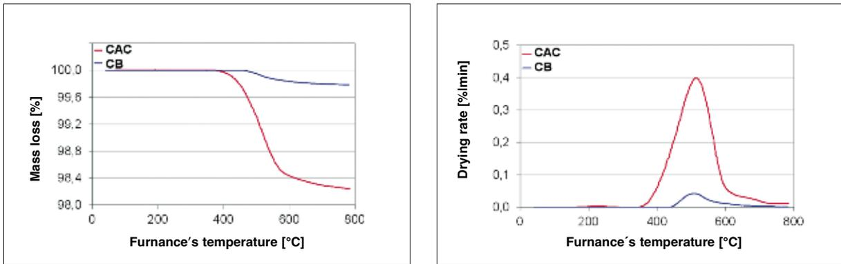
**Fig. 3** Drying behavior of cement-bonded (CAC) or colloidal-bonded (CB) refractory castables up to 800 °C, after 1 day of drying at 50 °C
