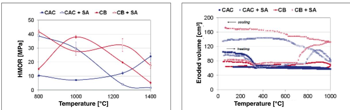
**Fig. 4** HMOR as a function of testing temperature (800–1400 °C) and elastic modulus evaluation up to 1000 °C for castables containing only cement (CAC) or only colloidal binder (CB) or bonded with these binders and containing sintering additive (CAC+SA or CB+SA)
