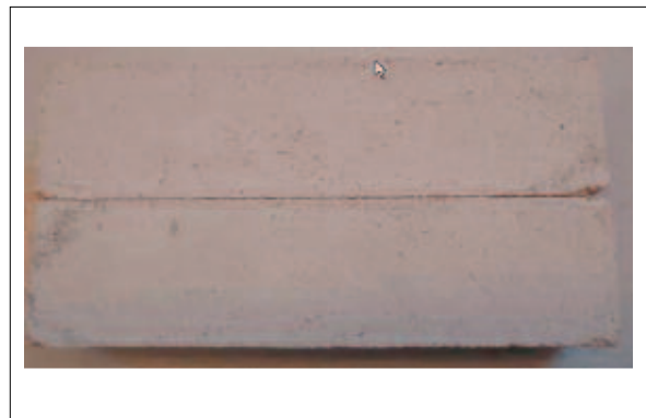
Fig. 6 Photo of cement-free MgO based castable with SioxX-Mag and microsilica
