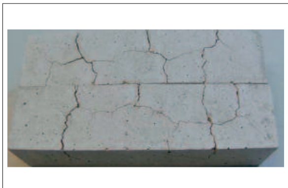
Fig. 7 Photo of cement-free MgO based castable without SioxX-Mag and without microsilica
