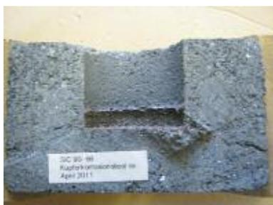
**Fig. 7** SiC crucible, copper test, oxidizing conditions: corrosion visible
