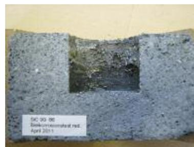
**Fig. 12** SiC crucible, lead test, reducing conditions: remarkable reduced corrosion
