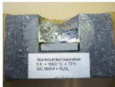
**Fig. 6** SiC crucible with Si<sub>3</sub>N<sub>4</sub> bottom disk after AlMg5-alloy test: no wetting
