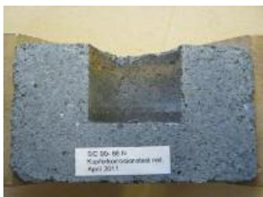
**Fig. 10** Nitrided SiC crucible, copper test, reducing conditions: no wetting
