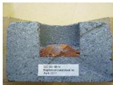
**Fig. 9** Nitrided SiC crucible, copper test, oxidizing conditions: only adherences of the metal
