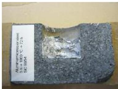
**Fig. 5** SiC crucible after test with AlMg5-alloy: just small infiltration
