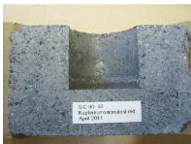
**Fig. 8** SiC crucible, copper test, reducing conditions: remarkable reduced corrosion
