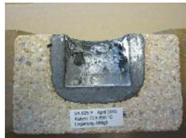
Fig. 1 Corundum formation in an andalusite based brick after test with AlMg5-alloy
