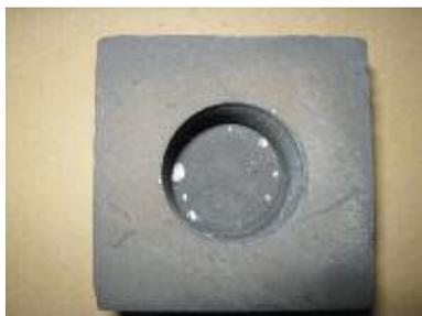
**Fig. 4** Pure carbon crucible after test with AlMg5-alloy: melt completely cast off after test
