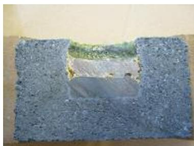
**Fig. 11** SiC crucible, lead test, oxidizing conditions: heavy corrosion, formation of lead oxides/silicates
