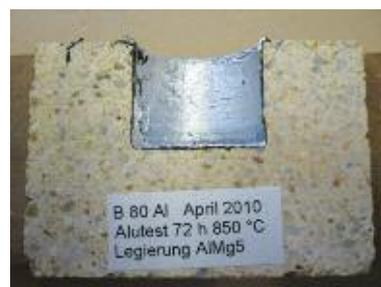
Fig. 2 Bauxite brick with high phosphate content after test with AlMg5-alloy
