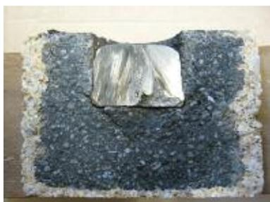
**Fig. 13** AC-brick crucible with  $\text{Si}_3\text{N}_4$  bottom disk, tested with steel 5 h 1500 °C: total disappearance of the  $\text{Si}_3\text{N}_4$
