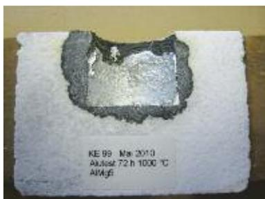
**Fig. 3** MgO/Spinel formation by the Mg-part of AlMg5-alloy after crucible test
