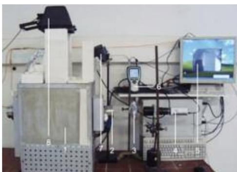
**Fig. 3** Test setup dynamic blistering test: SiC tube furnace; water cooled tube; black glass; CCD camera; user interface; ALMEMO-instrument; air cooler; lightning
