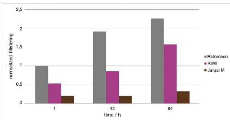
Fig. 4 Normalized blistering of the static blistering test at 1050 °C
