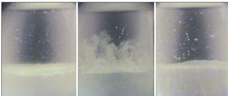
Fig. 6 Blistering of Jargal M (l.), reference Arkal 60PR (middle) and RW II (r.) after 12 h at 1050 °C
