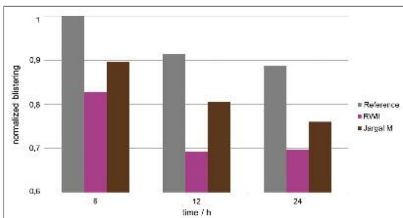
Fig. 5 Normalized blistering of the dynamic blistering test at 1050 °C
