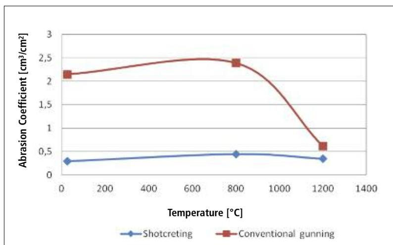
Fig. 3 Abrasion coefficient change of gunned samples at elevated temperatures
