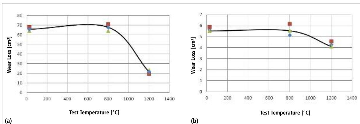
Fig. 2a–b Abrasion loss of samples by conventional gunning (a) and shotcreting (b) after hot abrasion test at elevated temperatures
