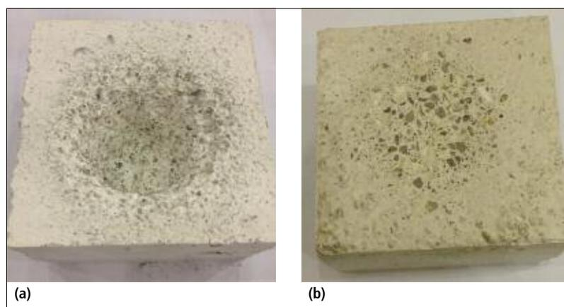
**Fig. 1a–b** The surface view of samples prepared by conventional gunning (a) and shotcreting (b) after the blast abrasion test at 25 °C after pre-firing at 1200 °C
