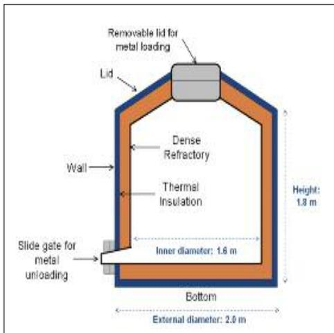
**Fig. 1** Schematic design of a molten aluminum transportation crucible [8]
