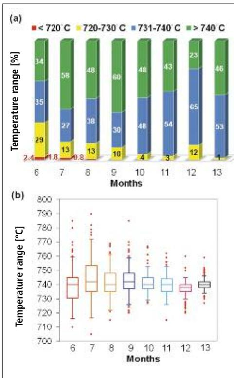
**Fig. 5a–b** Percentage of molten metal delivering temperatures for different temperature ranges, before (months 6 and 7) and after (8–13) process adjustments (a), and “box plot” evaluation of molten metal delivering temperatures (b)
