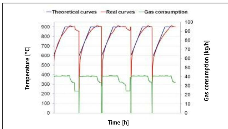
Fig. 4 Pre-heating curves (theoretical and real) of crucible No. 3 (5 years of operation), after establishing a new process procedure
