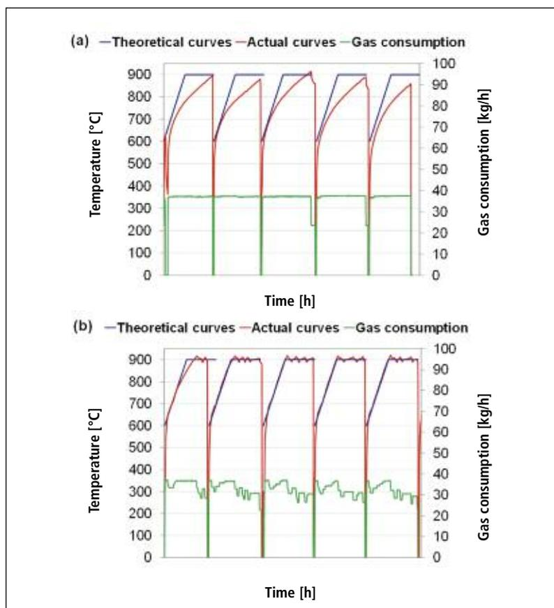
Fig. 3a–b Pre-heating curves (theoretical and actual) of: (a) crucible No. 3 (5 years of operation) and (b) crucible No. 4 (new refractory lining)
