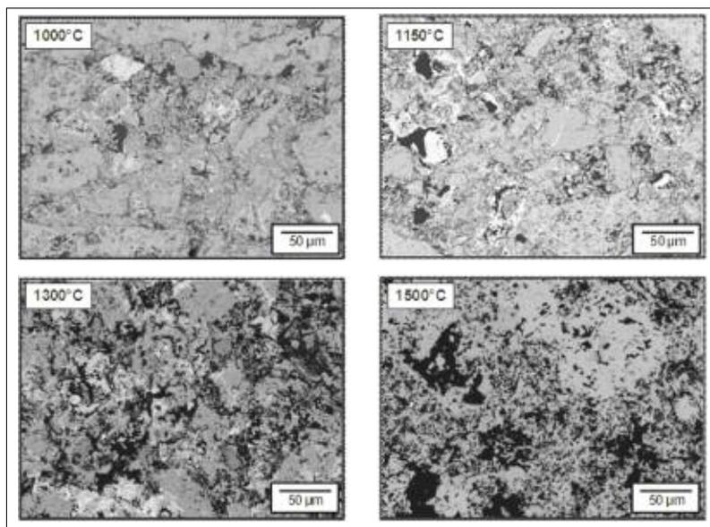
**Fig. 2** SEM images of alumina-magnesia castable containing MgO <45 μm after firing at 1000, 1150, 1300 and 1500 °C (APS = average pore size in the matrix)
