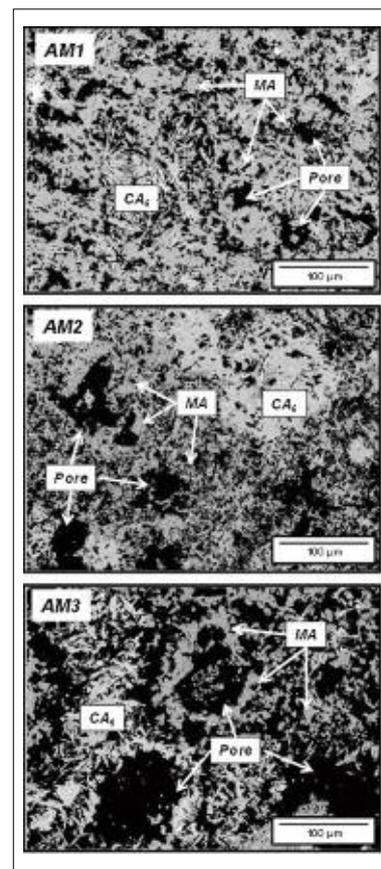
**Fig. 3** Microstructure of the castables AM1, AM2 and AM3 after firing at 1500 °C for 5 h
