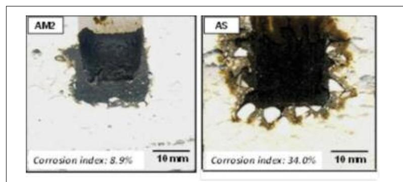
**Fig. 4** Cross sections and corrosion indexes of the samples containing *in situ* and pre-formed spinel after the corrosion tests
