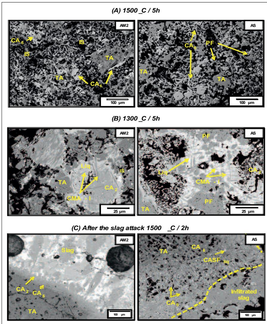
**Fig. 5** Microstructure of AM2 and AS castables fired at 1500 °C/5 h (A) and 1300 °C/5 h (B), and after the corrosion tests at 1500 °C/5 h (C). TA: tabular alumina; IS: *in situ* spinel; PF: pre-formed spinel
