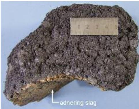
**Fig. 4** Post-mortem sample of the reference ramming mix after 14 days of application in the slag runner
