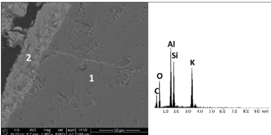
**Fig. 1** SEM micrograph of the reaction zone near the interface of the corroded  $\text{Al}_2\text{SiO}_5\text{-SiC}$  brick; 1 –  $\text{Al}_2\text{SiO}_5$ , 2 – KAlSiO<sub>4</sub> (Spot 2 – EDS analysis – Fig. 1a)
