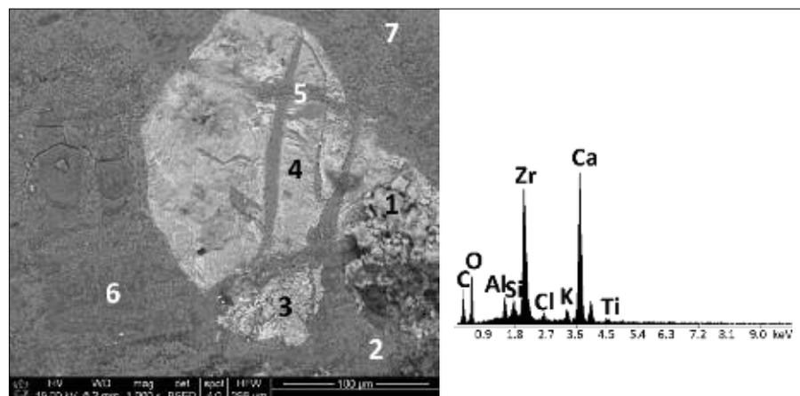
**Fig. 2** SEM backscatter image of the corroded  $\text{Al}_2\text{SiO}_5$ -ZrSiO<sub>4</sub> brick (interface); 1 – KCl, 2, 5, 7 –  $\text{Ca}_2\text{SiO}_4$ , 3 –  $\text{CaZrO}_3$  (Spot 3 – EDS analysis – Fig. 2a), 4 –  $\text{Ca}_3\text{ZrSi}_2\text{O}_9$ , 6 –  $\text{Ca}_{12}\text{Al}_{14}\text{O}_{33}\text{Cl}_2$
