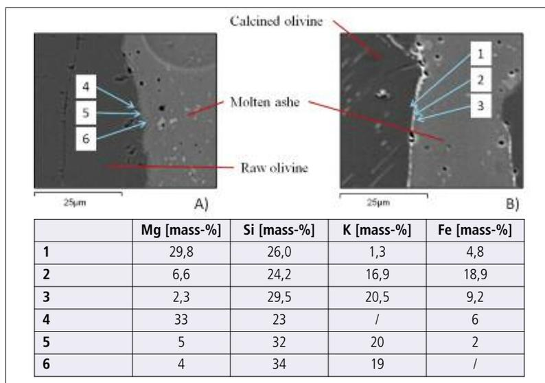
Fig. 5a–b SEM-EDX analysis showing the interactions between ash and a) natural olivine and b) calcined olivine
