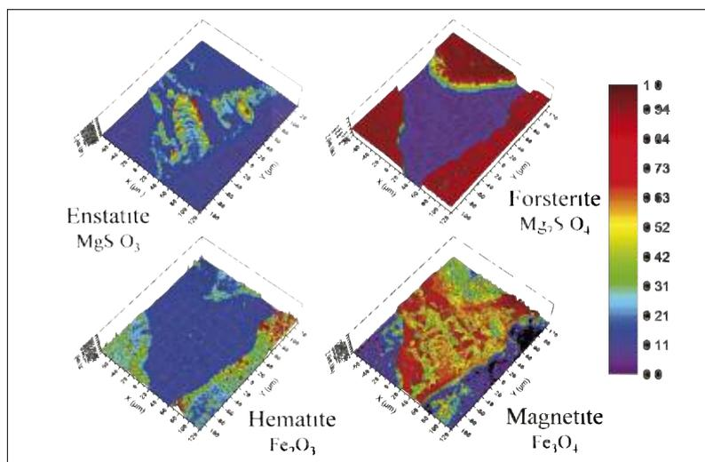
Fig. 4 Raman mapping of calcined olivine sintering
