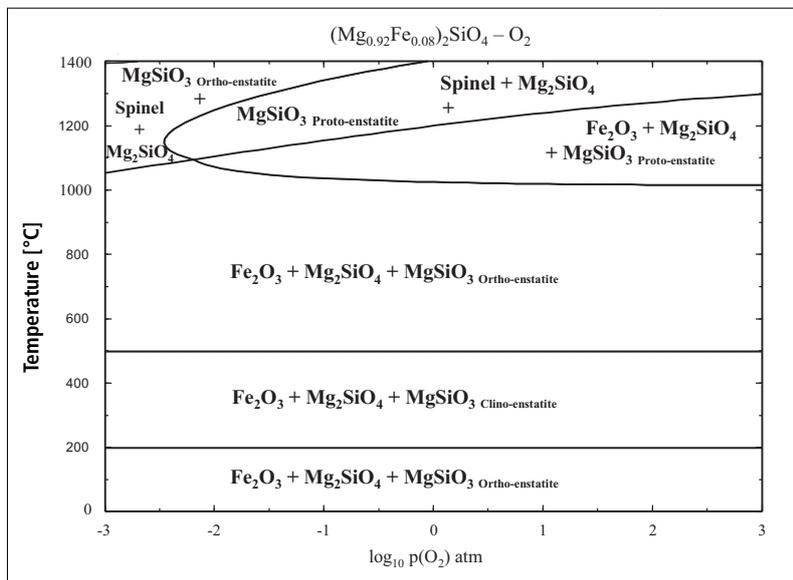
Fig. 2 Phase diagram of  $(Mg_{0.92}Fe_{0.08})_2SiO_4 - O_2$ , Factsage v6.2
