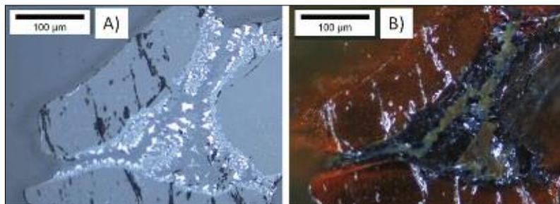
Fig. 3a–b Micrograph of calcined olivine at 1400 °C/48 h: a) bright field, b) dark field
