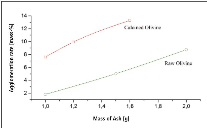
Fig. 7 Agglomeration test in fluidized bed reactor
