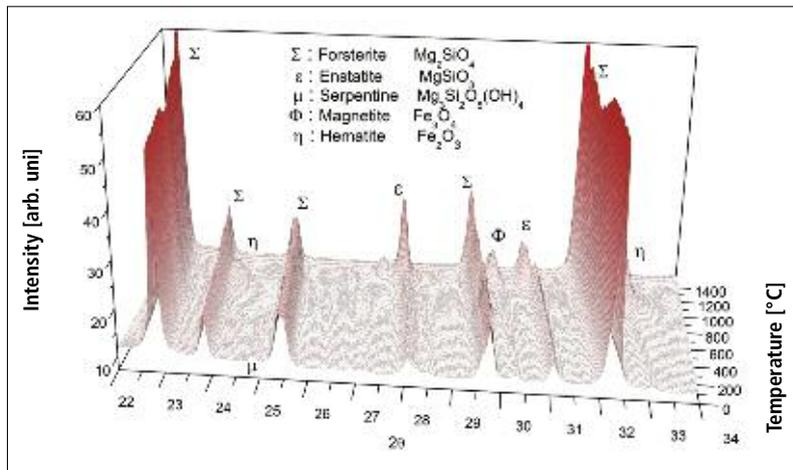
Fig. 1 In situ HT-XRD of olivine
