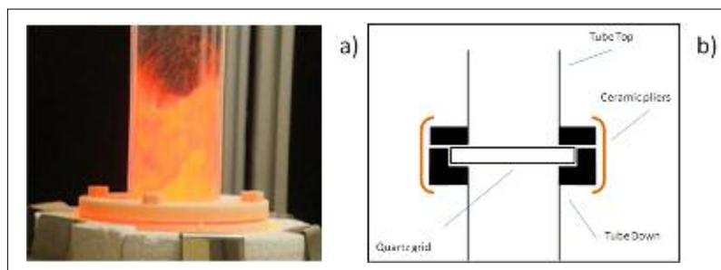
Fig. 6 Reactor made of quartz
