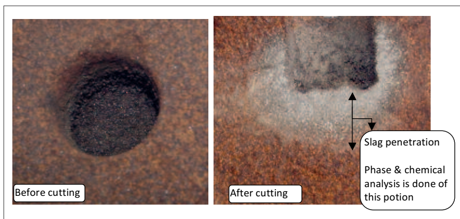
Fig. 1 Slag corroded DVM samples before and after cutting
