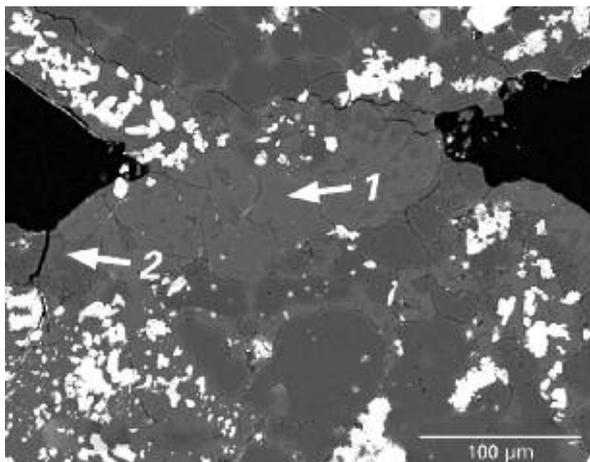
**Fig. 4** Magnesia-zircon brick sample that had undergone a laboratory corrosion test where the heating and cooling phases were under alternating reducing and oxidizing conditions, respectively. 96 cycles were performed between 800 °C and 1100 °C. Mainly sodium attack occurred. Newly formed Na-Mg-silicate (1), minimal Na-sulphur phases (2), corroded forsteritic matrix (3) with ZrO<sub>2</sub> (white), MgO (4), and pores (black) are indicated (source: RHI AG)
