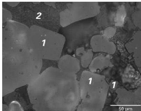
**Fig. 7** Pure magnesia brick after sulphate attack caused by an oxidizing atmosphere: precipitation of idiomorphic, cubic shaped MgO (1) from the sulphate melt (2) is visible (source: RHI AG)
