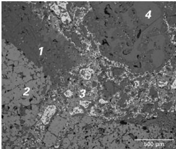
**Fig. 2** Magnesia-zircon checker brick after 17 years in service. At the near surface, up to a maximum of 5 mm from the hot face, corrosion of magnesia (2) due to the formation of a sulphate phase (1) is visible. The forsteritic matrix shows very high resistance against sulphate attack (3) and pores (4) are indicated (source: RHI AG)
