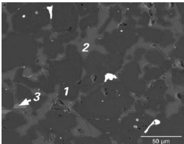
**Fig. 6** Pure magnesia brick, approximately 1,5 mm from the hot face brick, after sulphate attack caused by an oxidizing atmosphere: some residual MgO bonding bridges remain. MgO (1), Na-Mg-(K)-Ca-sulphate (2), and Ca-sulphate (3) are indicated. SEM-EDX analysis of point 2 detected 11,6 mass-% Na<sub>2</sub>O, 18,7 mass-% MgO, 66,0 mass-% SO<sub>3</sub>, 1,2 mass-% K<sub>2</sub>O, and 2,5 mass-% CaO (source: RHI AG)
