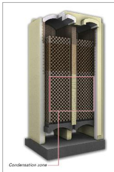
**Fig. 1** Glass tank regenerator: the condensation zone has a temperature range of approximately 700–1100 °C (source: RHI AG)
