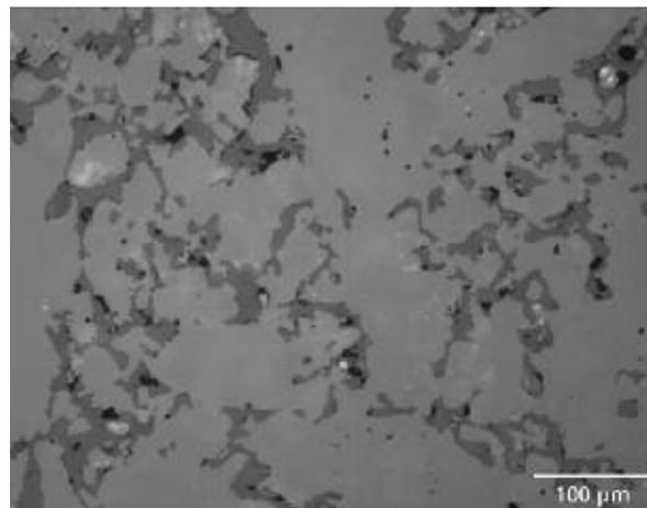
**Fig. 5** High fired pure magnesia brick.: the fines develop a strong bonding matrix (source: RHI AG)
