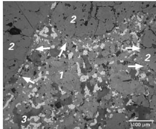
**Fig. 3** Microstructural detail 7 mm from the surface of a magnesia-zircon checker brick after 17 years in service: no corrosion of the forsteritic bonding matrix (1). The forsteritic belt (arrows) protecting the magnesia grains (2) and Na-Mg-sulphate in the pores (3) are indicated (source: RHI AG)
