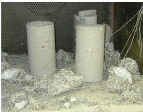
**Fig. 2 Explosive spalling of high performance concrete (Noumowe et al. [7])**
