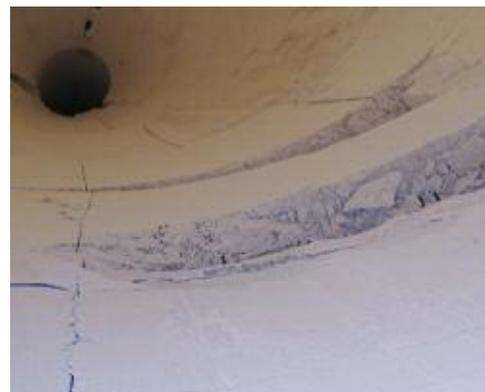
**Fig. 1** View of exploded refractory panel (LCC), which occurred during dryout
