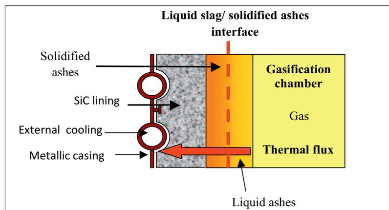
**Fig. 2** Refractory structure composed of SiC lining and metallic casing
