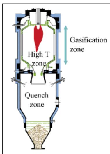
**Fig. 1** Biomass entrained flow reactor
