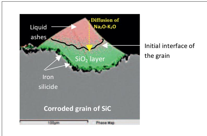
**Fig. 8** Silica-rich layer at the interface SiC grain/liquid ashes
