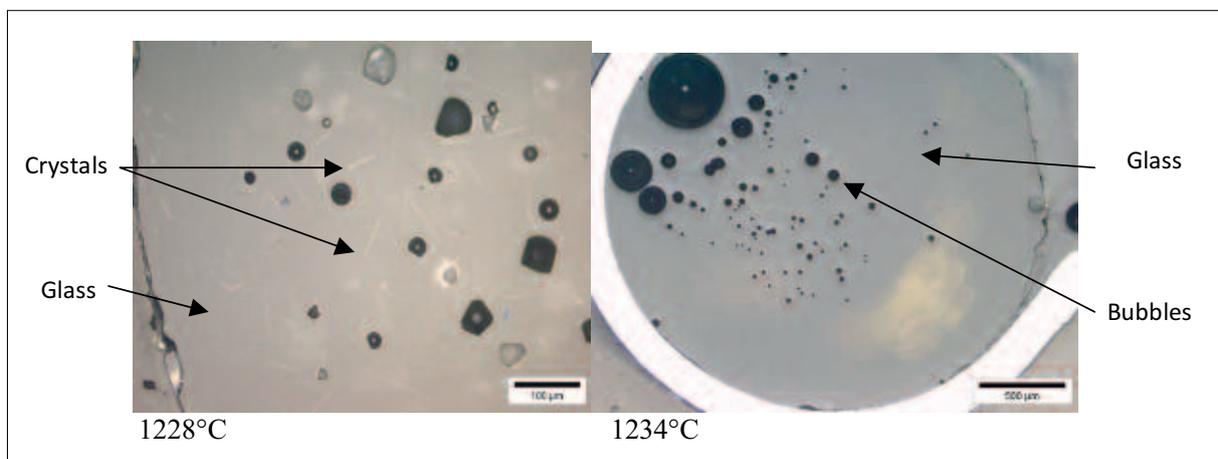
**Fig. 5** Microstructure of miscanthus ash quenched at 1228 and 1234 °C respectively, with sealed capsule
