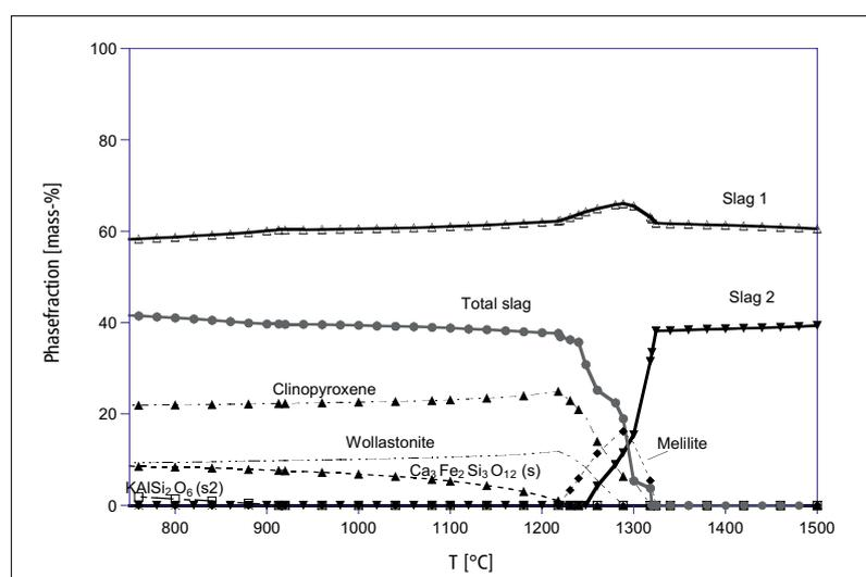
**Fig. 3** Phases formed [mass-%] as a function of the temperature for miscanthus ashes
