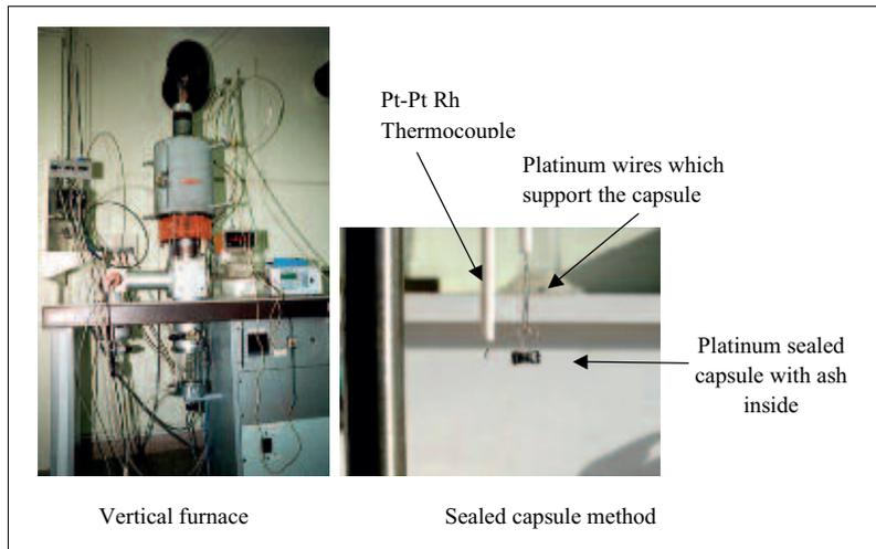
**Fig. 4** Quenching furnace
