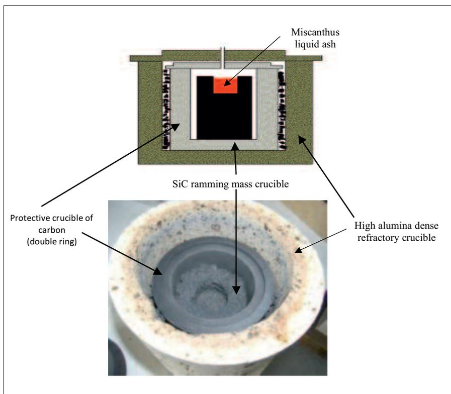
**Fig. 6** Detail of the corrosion apparatus and view of the SiC ramming mass crucible
