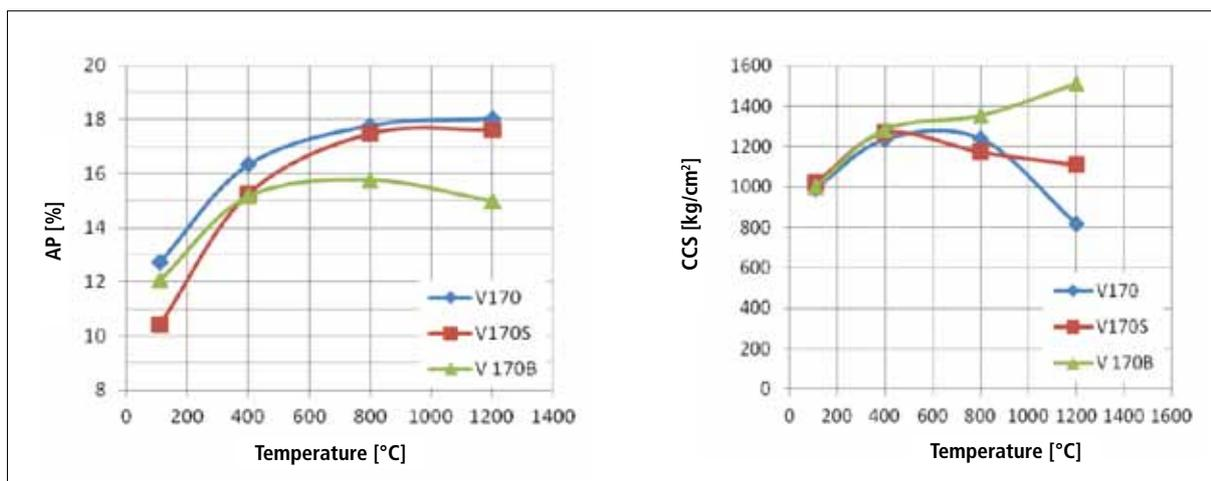
**Fig. 1** AP and CCS values of castable after firing at different temperatures
