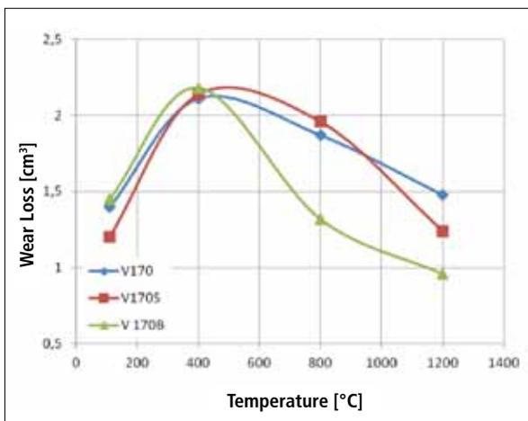
**Fig. 4** In situ hot abrasion loss of samples at different temperatures
