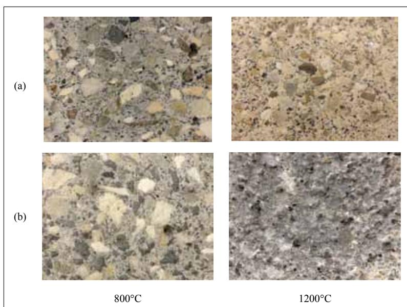
**Fig. 2** The eroded surface view of V 170S (a) and V 170 B (b) samples after hot abrasion test at 800 °C and 1200 °C
