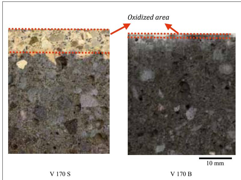
**Fig. 3** Cross section views of samples after blast abrasion test at 1200 °C
