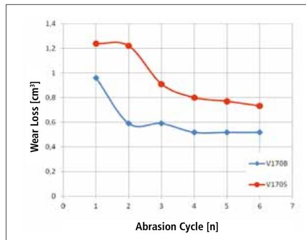
**Fig. 5** Hot abrasion loss of samples with abrasion cycles at 1200 °C
