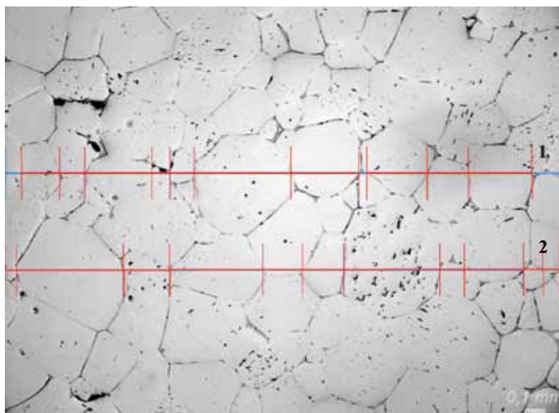
**Fig. 1** A site of fused periclase; size of separate crystals, found out in the microscope eyeglass field, was evaluated by method of intersected lines (chords). Reflected light; magnification: 25 $\times$ . Section lines were chosen for measuring 1 and 2.
