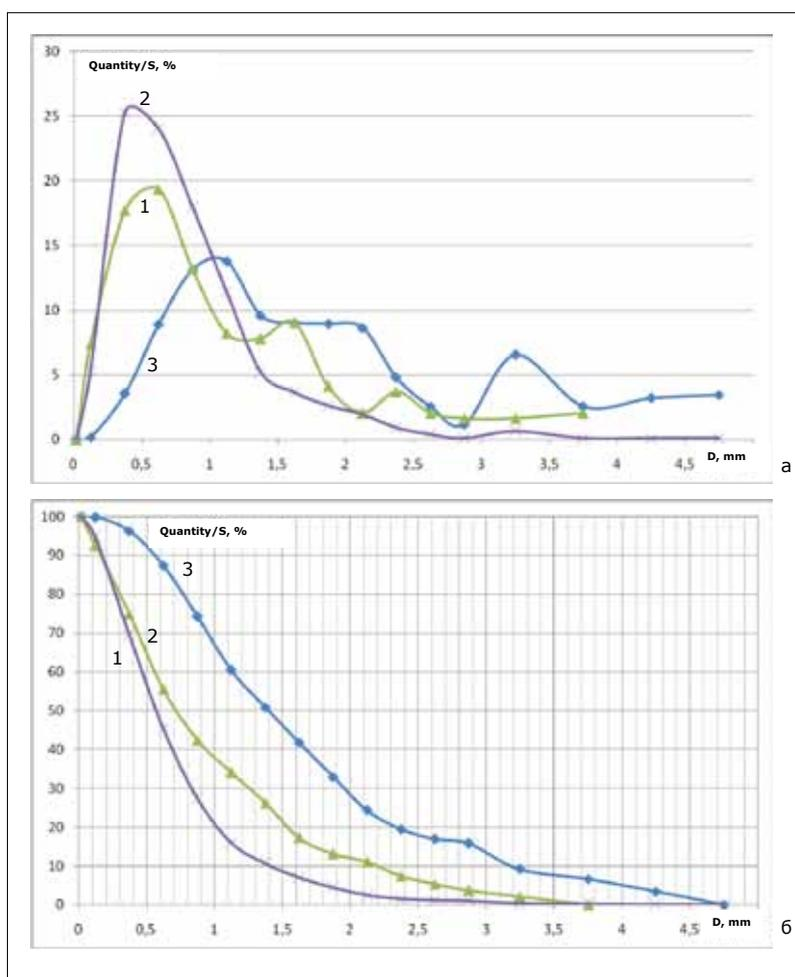
**Fig. 4 a–b** Curves of distribution of crystal sizes in fused periclase: **a** – differential curve of distribution of crystal sizes, **b** – integral curve of distribution of crystal sizes. 1 – old method of chords, 2 – new method of general analysis, distribution by number of crystals, 3 – new method of general analysis, distribution along the surface of crystals
