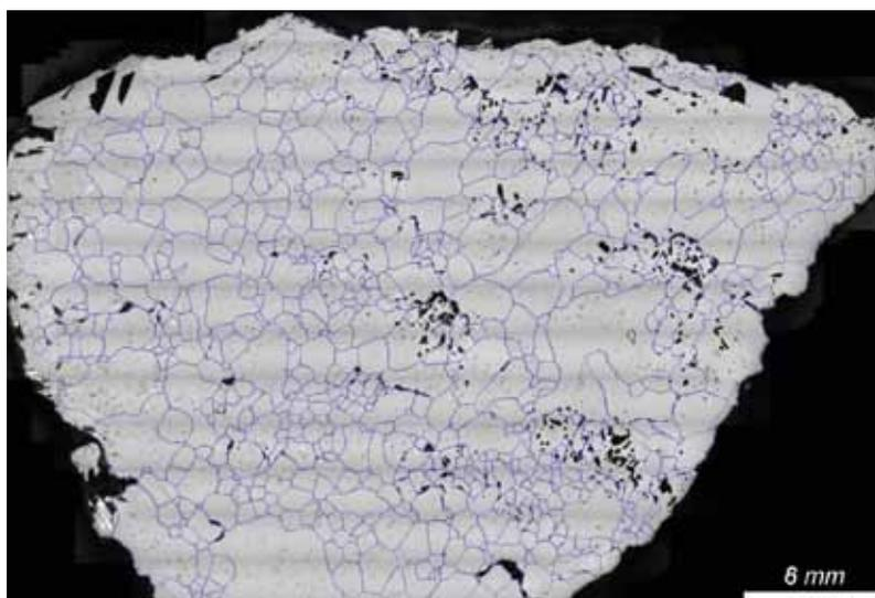
**Fig. 2** Example of assessment of the surface of periclase crystals along the whole surface of polished section. Reflected light; magnification: 4×
