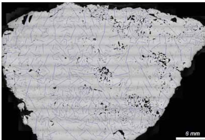
**Fig. 3** Example of assessment of the surface of periclase crystals along the whole surface of polished section. Reflected light; magnification: 4×
