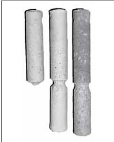
**Fig. 1** Samples after 96-h finger test at 1475 °C: AZS – porous, AZS – fused cast and AZS – porous with surface treatment technology (from left to right)
