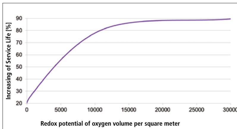
**Fig. 2** Influence of the oxygen depression on the service life of the refractory material
