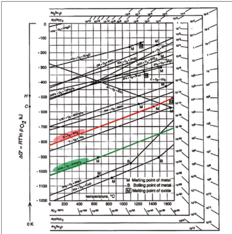
**Fig. 1** The Jeffes-Richardson-Diagramm [10] shows the enthalpy of formation  $\Delta G$  as a function of temperature. It describes the thermodynamic stability of oxides, which increases with lower  $\Delta G$  values. It is known that  $\text{SiO}_2$  (red graph) is reduced by the presence of molten aluminum.
