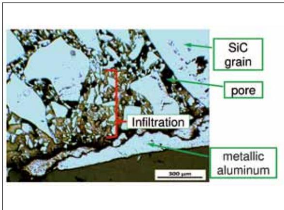
Fig. 9 LM-micrograph of Al-test of SC 90
