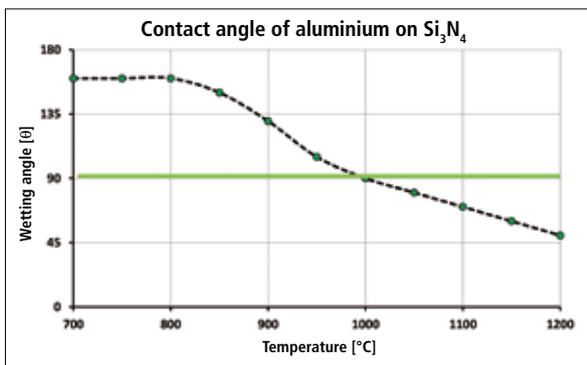
**Fig. 4** Wetting angle  $\theta$  as a function of temperature [11]. The transition from non-wetting to wetting ( $\theta = 90^\circ$ ) is for Si<sub>3</sub>N<sub>4</sub> at about 1000 °C.
