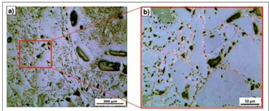
**Fig. 15 LM-micrograph of Al-test of K 99 (850 °C, 72 h)**
