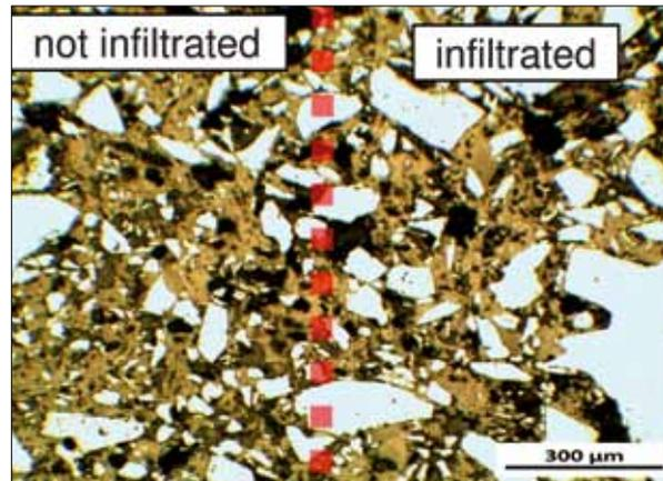
Fig. 10 LM-micrograph of Al-test of SCN 70 (1100 °C, 72 h)
