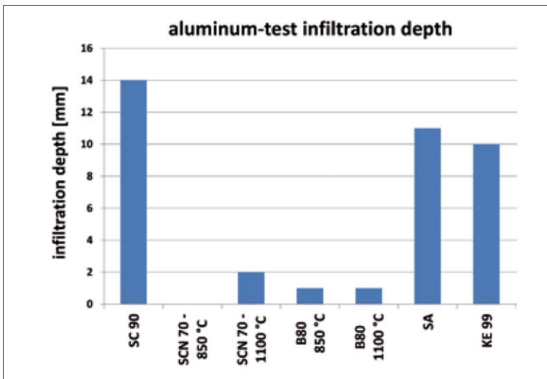
aluminum on  $\text{Si}_3\text{N}_4$  substrates confirms the test results (Fig. 4). The critical temperature ( $\theta < 90^\circ$ ) of  $\text{Si}_3\text{N}_4$  is estimated to be about 1000 °C.
