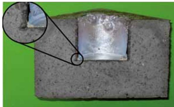
**Fig. 5** Al-crucible test of SCN 70, dwelling time: 72 h, temperature: 1100 °C
