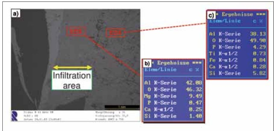
**Fig. 13 SEM and EDX analysis of B 80 Al-test (850 °C):**
