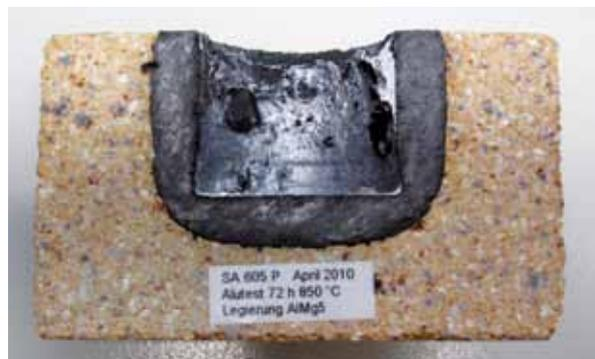
**Fig. 7** Al-crucible test of SA, dwelling time: 72 h, temperature: 850 °C
