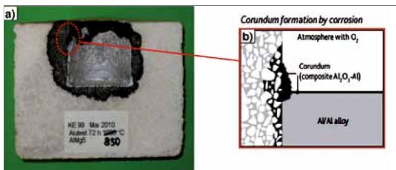
**Fig. 8** Al-crucible test of K 99, dwelling time: 72 h, temperature: 850 °C, schematic of the „corundum growth“ [8]
