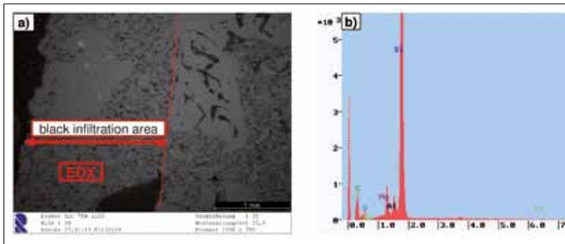
Fig. 11 SEM and EDX analysis of SCN 70 Al-test:
