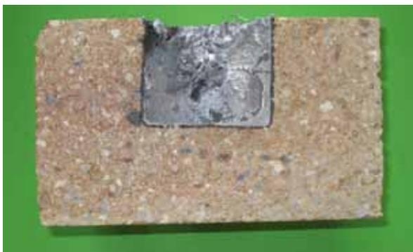
**Fig. 6** Al-crucible test of B 80, dwelling time: 72 h, temperature: 850 °C
