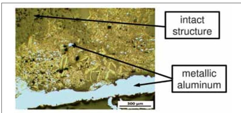
Fig. 12 LM-micrograph of Al-test of B 80 (1100 °C, 72 h)
