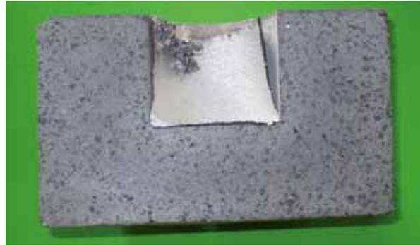
**Fig. 3** Al-crucible test of SCN 70, dwelling time: 72 h, temperature: 850 °C
