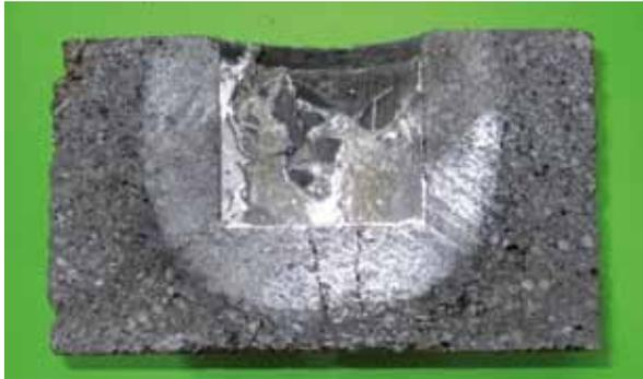
**Fig. 2** Al-crucible test of SC 90, dwelling time: 72 h, temperature: 850 °C
