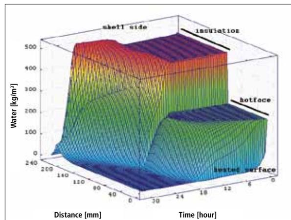
**Fig. 7** Water content with time and thickness – 50 °C/h with 10 h hold at 125 °C
