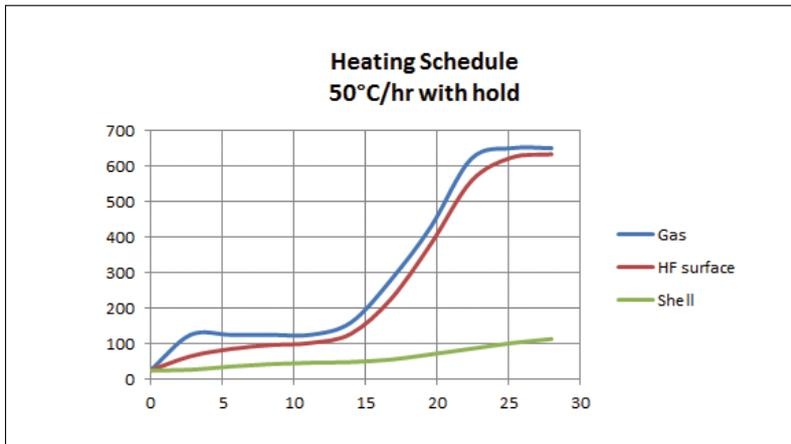
**Fig. 5** Heating schedule showing lag between the gas temperature and refractory surface temperature
