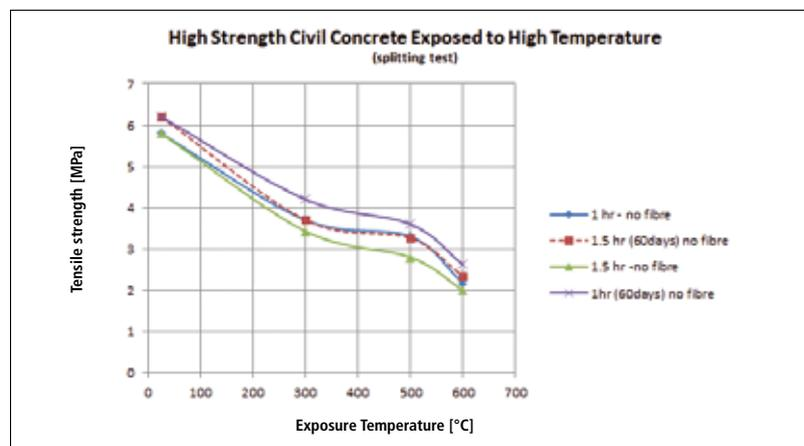
Fig. 4 Variation in hot tensile strength with temperature for high strength concrete [10]
