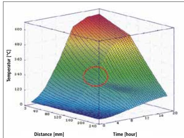
**Fig. 9** Temperature with time and thickness – 50 °C/h with no hold
