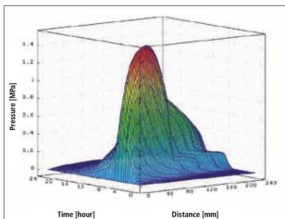
**Fig. 15** Pore pressure with time and thickness. Max. pressure reached was ~1,49 MPa at ~6 h at depth of ~60 mm – 100 °C/h with no hold.
