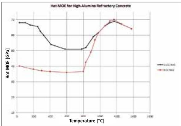
Fig. 2 Variation in hot elastic modulus for low cement and no-cement refractory concrete [12]
