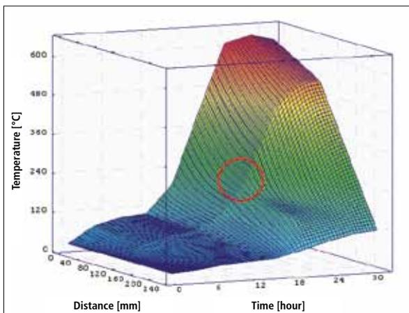
**Fig. 6** Temperature with time and thickness – 50 °C/h with hold at 125 °C
