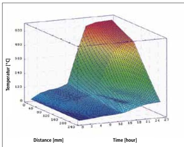
**Fig. 12** Temperature with time and thickness – 100 °C/h with hold at 125 °C
