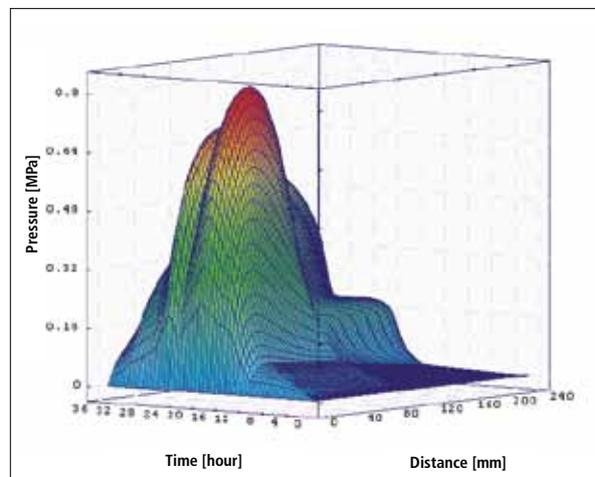
**Fig. 18** Vapour pressure graph showing peak pressure for heating at 50 °C/h, first hold at 125 °C and second hold period at 300 °C for 7 h – peak pressure is ~0,82 MPa at 20,5 h at depth of ~57 mm
