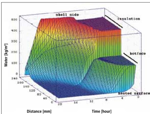
**Fig. 10** Water content with time and thickness – 50 °C/h with no hold
