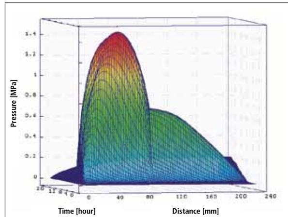
**Fig. 17** Vapour pressure graph showing peak pressure for heating 100 °C/h, no hold and zero mass flow at the cold face – peak pressure is ~1,48 MPa at 5,7 h at depth of ~55 mm
