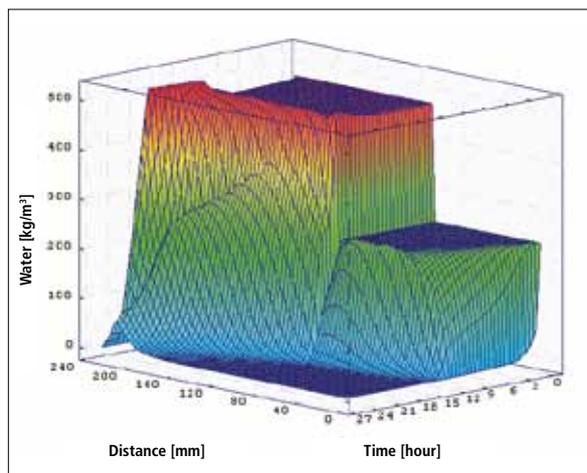
**Fig. 13** Water content with time and thickness – 100 °C/h with hold at 125 °C
