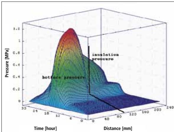
**Fig. 8** Pore pressure with time and thickness. Max. pressure reached was ~1,25 MPa at ~19,5 h at depth of ~60 mm – 50 °C/h with 10 h hold at 125 °C
