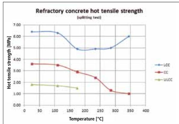
Fig. 3 Variation in hot tensile strength with temperature for different refractory concrete [13]
