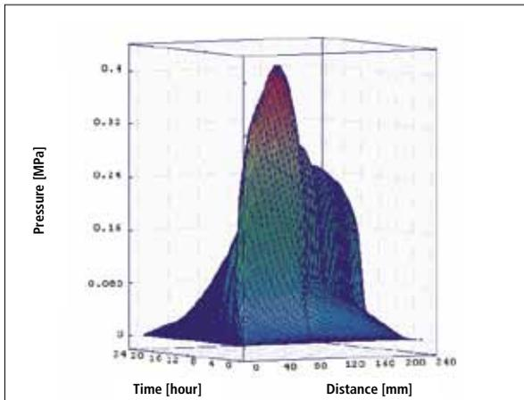
**Fig. 16** Pore pressure with time and thickness with hotface permeability equal to 0,1 % polypropylene fibre content. The peak pore pressure was ~0,42 MPa at 4,83 h and depth of ~68 mm – 100 °C/h with no hold.
