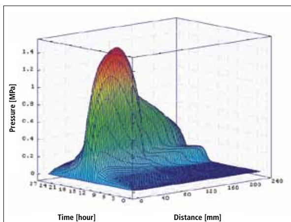
**Fig. 14** Pore pressure with time and thickness. Max. pressure reached was ~1,49 MPa at ~15,5 h and depth of ~60 mm – 100 °C/h with 10 h hold at 125 °C
