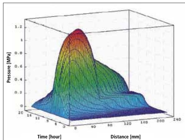
**Fig. 11** Pore pressure with time and thickness. Max. pressure reached was ~1,26 MPa at ~9 h and depth of ~60 mm – 50 °C/h with no hold
