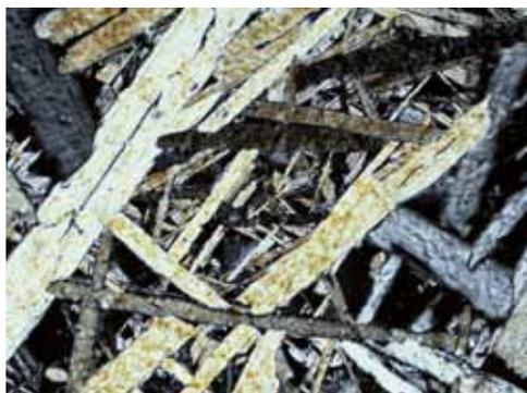
**Fig. 1** The structure of synthetic fluorphlogopite using an optical polarization microscopy ( $\times 150$ )
