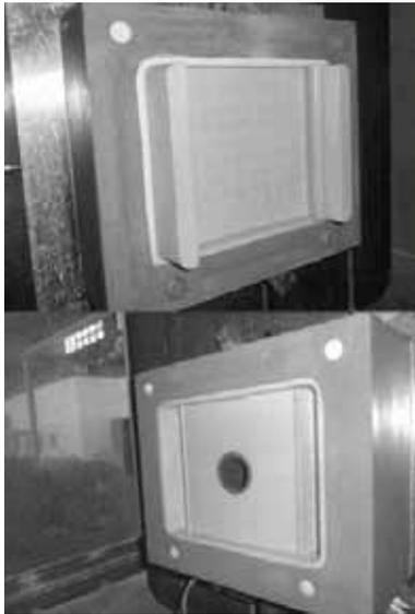
**Fig. 1** Quartered mould for heat shields
