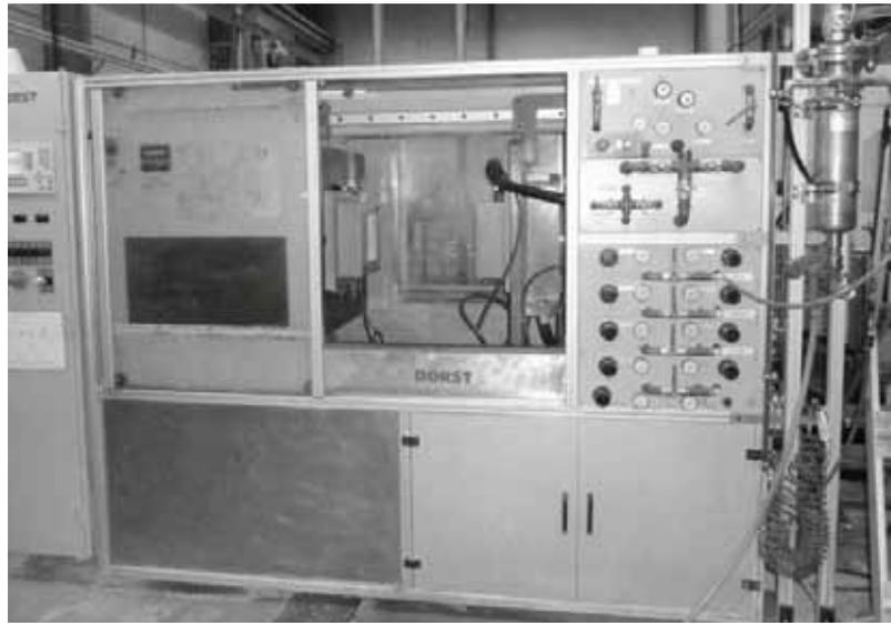
**Fig. 2** Pressure slip casting machine DGM-80D from DORST/DE
