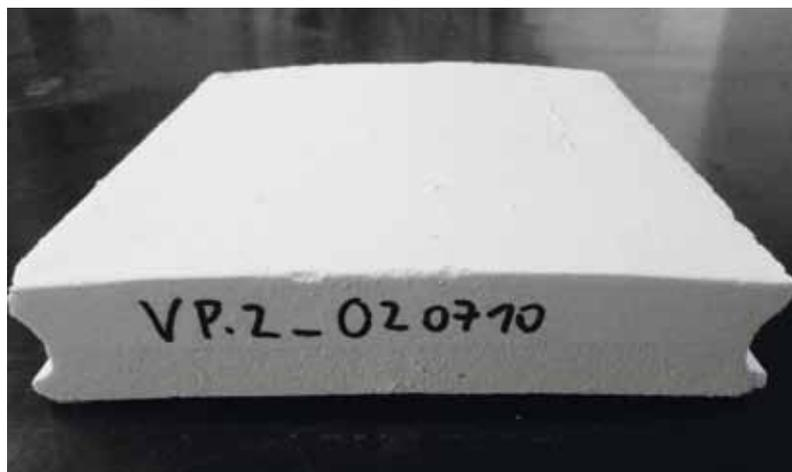
**Fig. 3** Heat shield made by pressure slip casting
