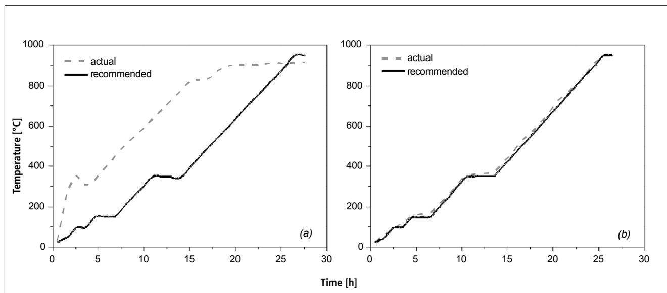
**Fig. 4** Heating profile for castable's drying (a) before and (b) after improvements in the pre-heating system of molten aluminum crucibles
