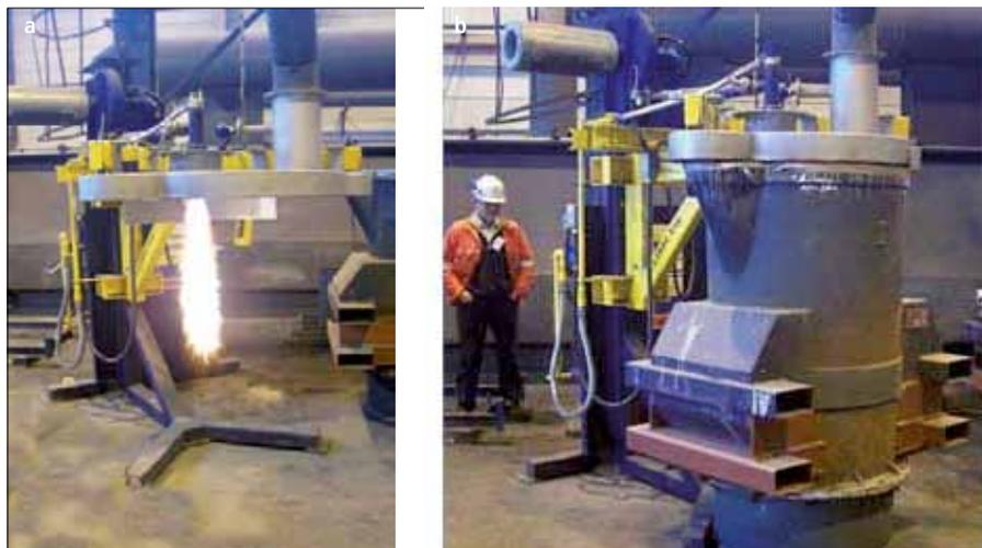
**Fig. 1** Gas-powered pre-heater in operation (a) without and (b) with a crucible
