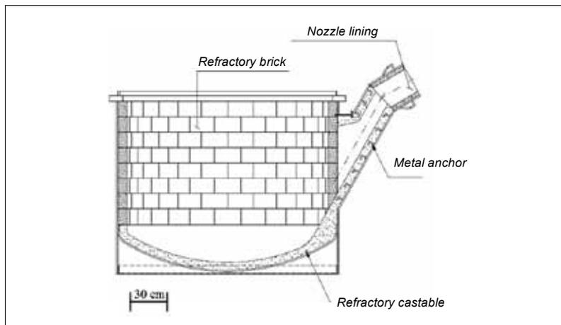
**Fig. 3** Sketch of a crucible used at Alcoa plant in Poços de Caldas (Brazil), highlighting the shaped (bricks) and castable refractories lining this equipment
