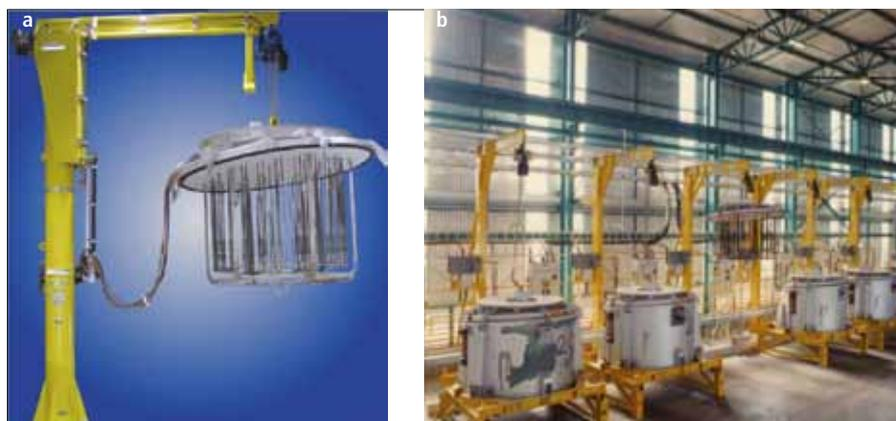
**Fig. 2** Electric pre-heater (a) before and (b) during operation with crucibles
