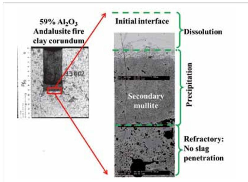
Fig. 3 SEM microstructure (back scattered electron) of final corrosion interface for andalusite/fireclay castable
