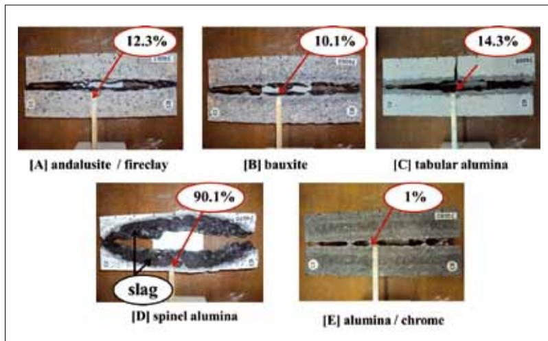
Fig. 2 Key brick after dynamic corrosion test
