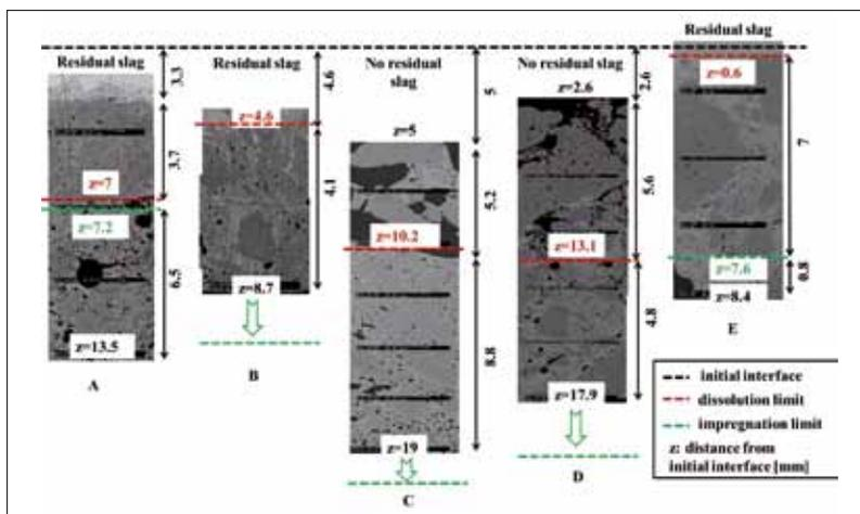
**Fig. 1** SEM (bse mode) microstructures of corroded area after isothermal test at 1500 °C during 5 h
