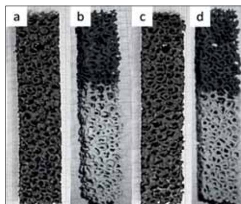
**Fig. 9** Samples before and after dipping into the steel melt at 1640 °C: (a) SS-C fine coked at 800 °C; (b) SS-C fine after dipping; (c) AR-C fine coked at 800 °C; (d) AR-C fine after dipping [14]
