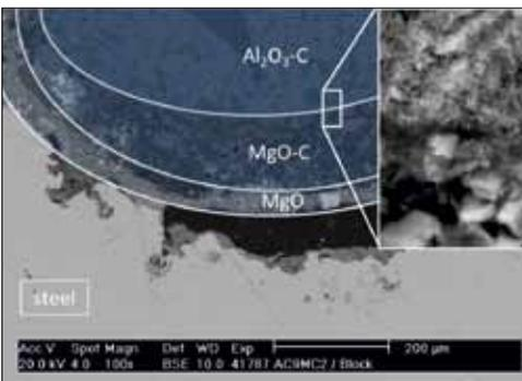
**Fig. 7** SEM image of filter AC9MC2 after passing the impingement test at 1670 °C [15]
