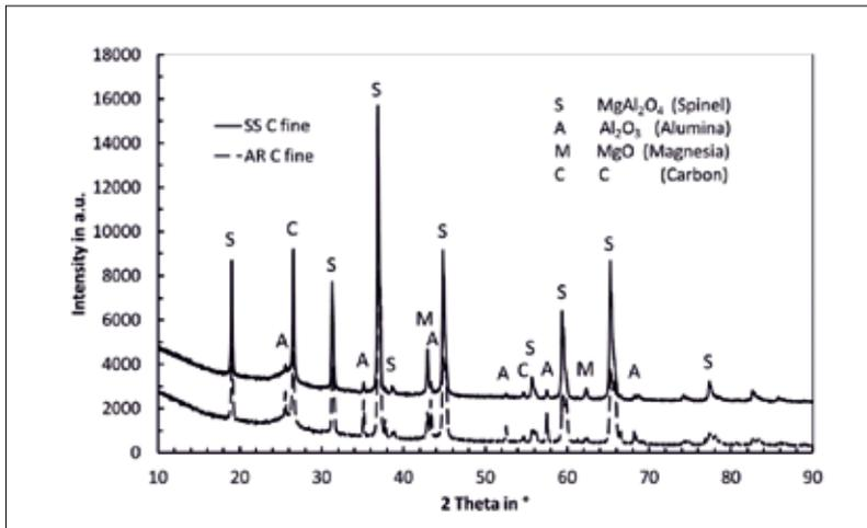
**Fig. 10** Phase evolution for samples AR-C fine and SS-C fine after dipping in the steel melt at 1640 °C [14]
