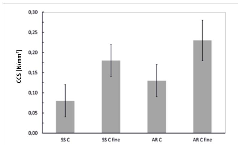
**Fig. 8** Cold crushing strengths of 10 ppi filters produced using particles of different size, after a thermal treatment at 800 °C [14]
