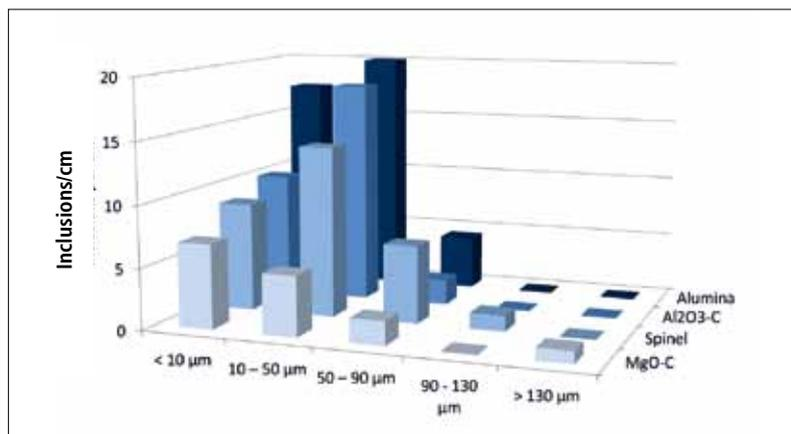
Fig. 12 Amount of trapped exogenous spinel as a function of filter chemistry [15]
