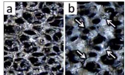
**Fig. 1 Resin coated, coked filters with (a) and without (b) thermal pretreatment at 800 °C [15]**
