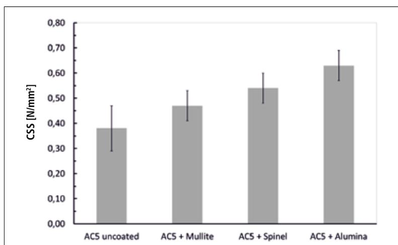
**Fig. 4** Cold crushing strengths of the coated and uncoated filter systems, coked at 1400 °C [12]
