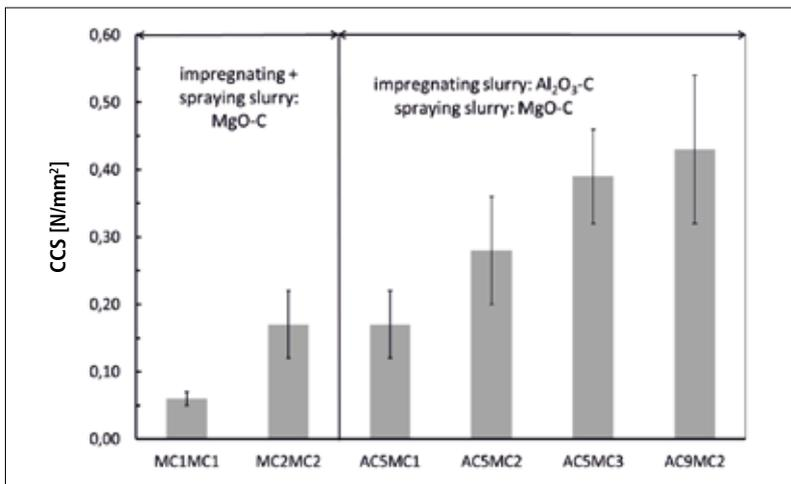
**Fig. 6** Cold crushing strengths of the reactive filters, consisting of different layer compositions [13]
