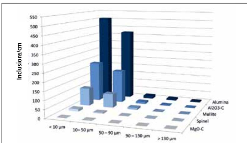
**Fig. 11** Amount of trapped exogenous alumina as a function of filter chemistry [17]
