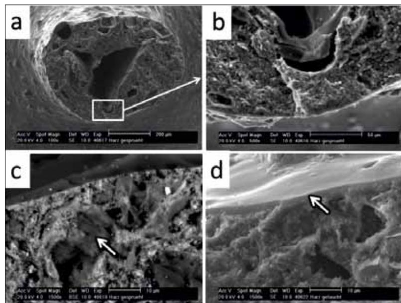
**Fig. 2 Resin coating of filter AC5 leads to rounding of the sharp edges of the hollow filter struts (a+b), reduction of the total open porosity (c) and increase of the load bearing cross section (d) [15]**
