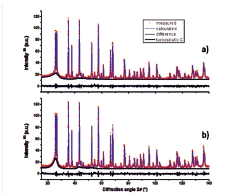
**Fig. 3** Measured (dots), refined (lines) and difference (lines at the bottom of each plot) X-ray diffraction patterns of specimens coked at 800 °C (a) and 1400 °C (b). The Carbores® P and carbon black contribution to the diffraction patterns (noted as turbostratic C) is shown as a thick line below the sharp crystalline phase's peaks [15]
