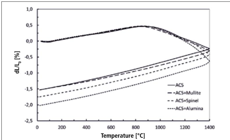
**Fig. 5** Shrinkage behavior of the coated and uncoated filters, in situ sintered under argon within the dilatometer [12]
