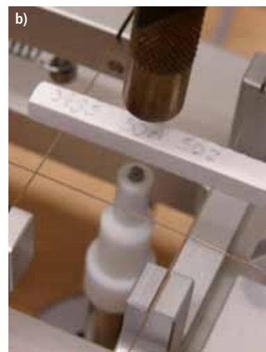
**Fig. 1 a)** Flexural mode experimental set up for the determination of elastic properties; **b)** overview of the measuring principle and the tested sample geometry (sample based on 50 % Al<sub>2</sub>O<sub>3</sub> and 50 % ZrO<sub>2</sub>)
