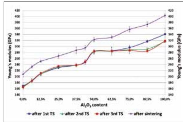
**Fig. 3** Evolution of the retained Young's modulus of tested formulations in function of the alumina content after progressive thermal shock cycles
