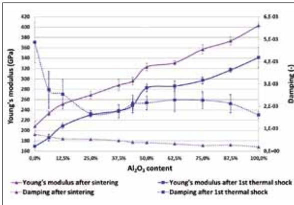
**Fig. 4** Evolution of the Young's modulus and the damping behaviour of the tested formulations after the first thermal shock cycle
