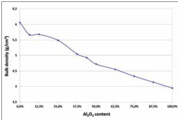
**Fig. 2** Evolution of the bulk density of the tested formulations according to the alumina content
