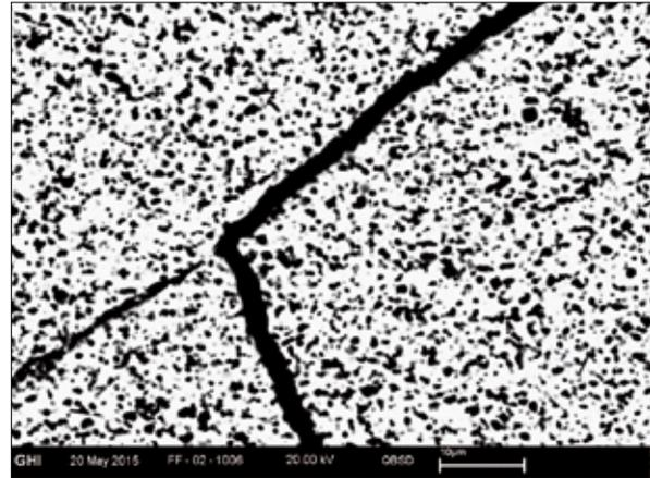
**Fig. 9** Crack propagating throughout the matrix of a sample based on 25 % alumina and 75 % zirconia after thermal shock test in water
