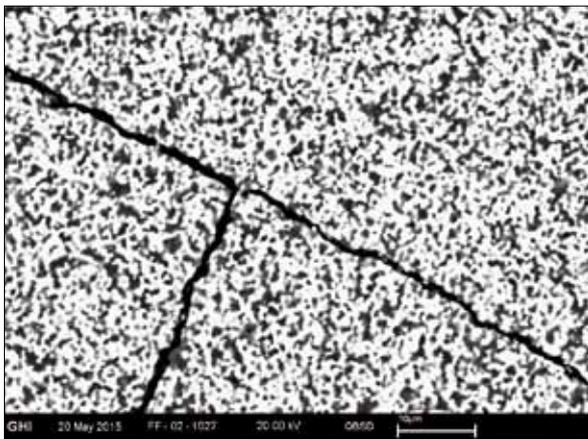
**Fig. 10** Crack branching or crack unification in the matrix of a sample based on 50 % alumina and 50 % zirconia after thermal shock test in water
