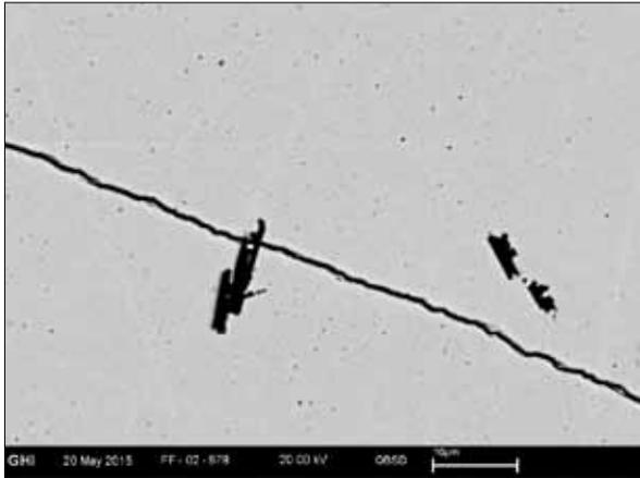
**Fig. 8** Crack crossing over a pore in a pure zirconia sample after thermal shock test in water
