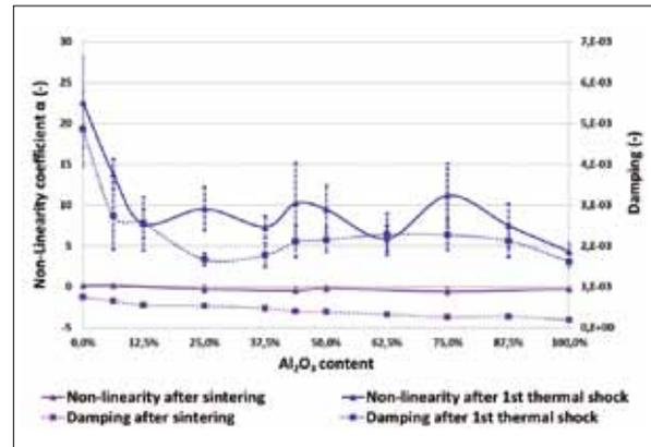
**Fig. 5** Evolution of non-linearity of the flexural resonant frequency and damping behaviour evolution after the first thermal shock cycle
