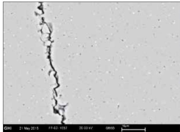
**Fig. 11** Crack propagation throughout the matrix of a pure alumina sample after thermal shock test in water
