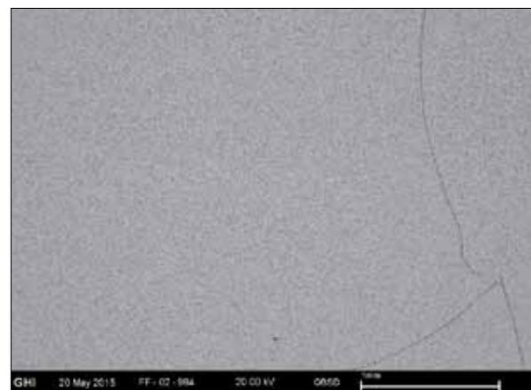
**Fig. 7** Overview of microstructural damaging of sample based on 6,25 % alumina and 93,75 % zirconia after thermal shock test in water
