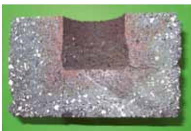
**Fig. 28** Pb-crucible test of CZK 15 in reducing atmosphere
