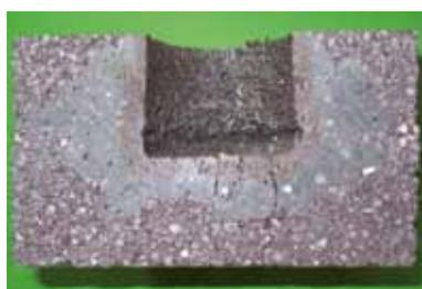
**Fig. 23** Pb-crucible test of CZK 5 in reducing atmosphere
