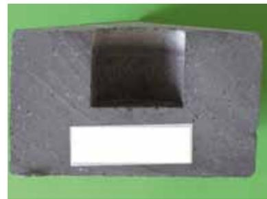
**Fig. 18** Cu-crucible test of SCN 70 in reducing atmosphere
