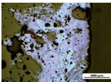
**Fig. 12** LM-micrograph of Cu-test of CZK 15 in reducing atmosphere
