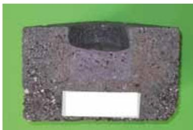
**Fig. 9** Cu-crucible test of CZK 15 in oxidizing atmosphere
