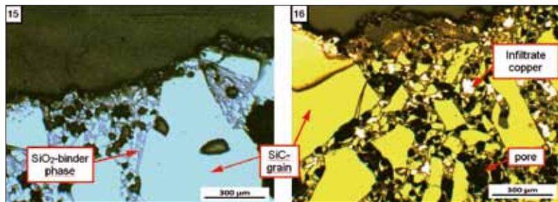
**Fig. 15–16** LM-micrograph of Cu-test of SC 90 in reducing atmosphere
