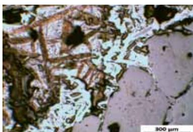
**Fig. 25** LM-micrograph of Pb-test of CZK 5 in oxidizing atmosphere
