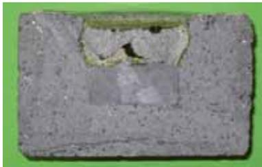
**Fig. 36** Pb-crucible test of SCN 70 in oxidizing atmosphere
