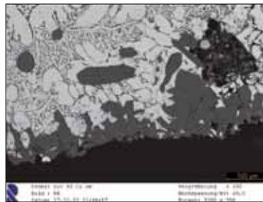
**Fig. 17** SEM of Cu-test of SC 90 in oxidizing atmosphere
