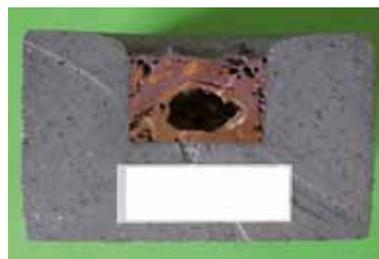
**Fig. 19** Cu-crucible test of SCN 70 in oxidizing atmosphere
