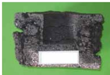
Fig. 1 Cu-crucible test of CK 9 in oxidizing atmosphere
