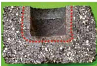
**Fig. 10** Cu-crucible test of CZK 15 in reducing atmosphere
