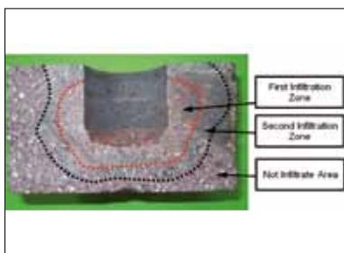
**Fig. 7** Cu-crucible test of CZK 5 in reducing atmosphere
