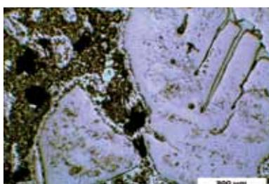
**Fig. 31** LM-micrograph of Pb-test of CZK 15 in reducing atmosphere
