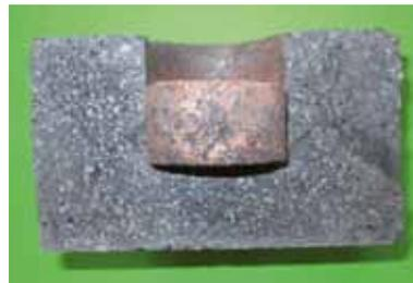
**Fig. 13** Cu-crucible test of SC 90 in reducing atmosphere
