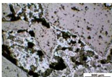
**Fig. 32** LM-micrograph of Pb-test of CZK 15 in oxidizing atmosphere
