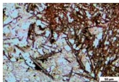
**Fig. 30** LM-micrograph of Pb-test of CZK15 in oxidizing atmosphere
