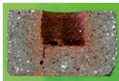
**Fig. 27** Pb-crucible test of CZK 15 in oxidizing atmosphere
