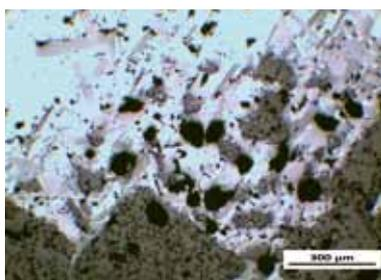
**Fig. 11** LM-micrograph of Cu-test of CZK 15 in oxidizing atmosphere
