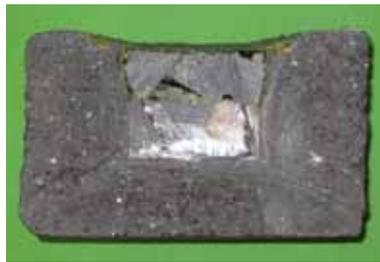
**Fig. 34** Pb-crucible test of SC 90 in oxidizing atmosphere
