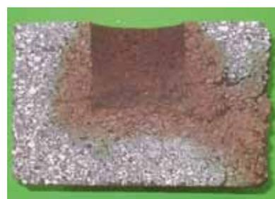
**Fig. 21** Pb-crucible test of CK 9 in reducing atmosphere
