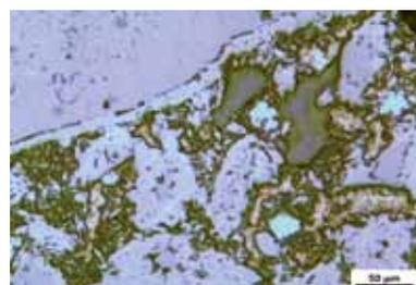
**Fig. 24** LM-micrograph of Pb-test of CZK 5 in reducing atmosphere
