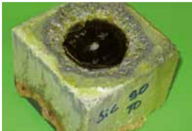
**Fig. 33** Pb-crucible test of SC 90 in oxidizing atmosphere
