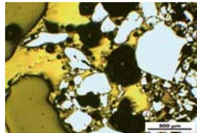
**Fig. 35** LM-micrograph of Pb-test of SC 90 in oxidizing atmosphere
