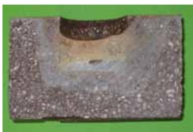
**Fig. 22** Pb-crucible test of CZK 5 in oxidizing atmosphere
