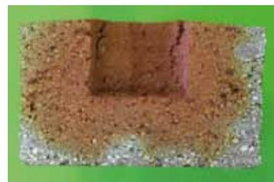
**Fig. 20** Pb-crucible test of CK 9 in oxidizing atmosphere
