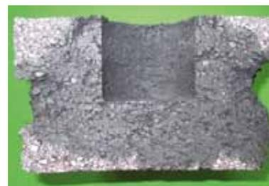
Fig. 2 Cu-crucible test of CK 9 in reducing atmosphere
