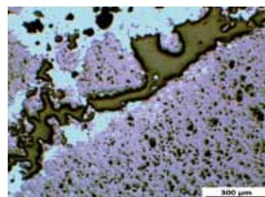
Fig. 4 LM-micrograph of Cu-test of CK 9 in oxidizing atmosphere
