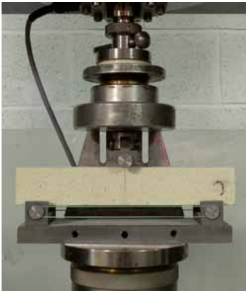
Fig. 3 Example of test jig used for the 3-point bending test of dense shaped specimens
