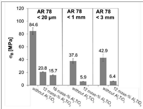
**Fig. 3** Three-point bending strength of the sintered bodies
