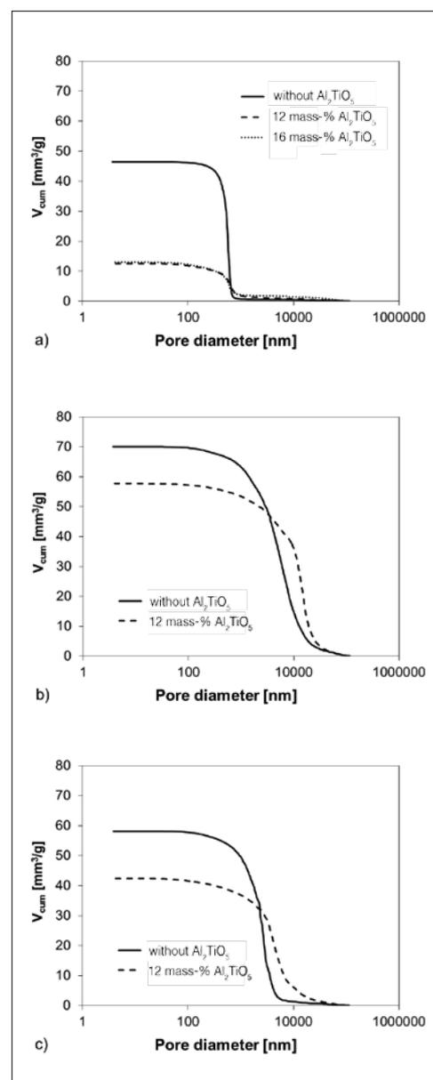
**Fig. 1 Cumulative pore volume vs. pore diameter of sintered bodies fabricated from raw materials with different maximum particle size: a) <20 µm, b) <1 mm, c) <3 mm**
