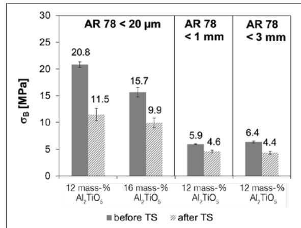
**Fig. 4** Three-point bending strength of the Al<sub>2</sub>TiO<sub>5</sub>-containing sintered bodies before and after quenching from 950 °C
