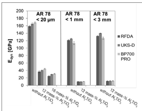
**Fig. 5** Dynamic Young's modulus determined after sintering by means of different methods and measuring systems: impulse excitation (RFDA) and ultrasonic testing (UKS-D, BP-700 Pro)
