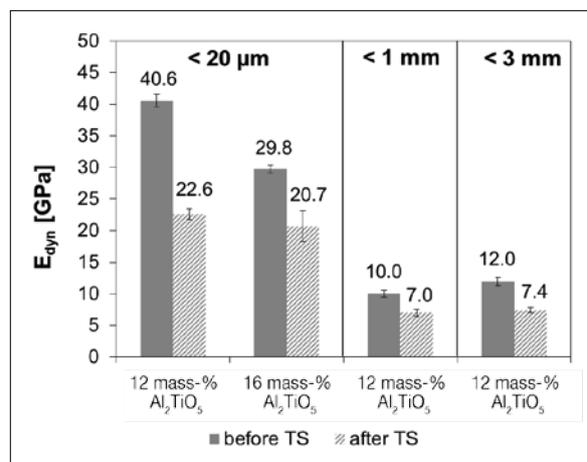
**Fig. 6** Dynamic Young's modulus of the Al<sub>2</sub>TiO<sub>5</sub>-containing sintered bodies before and after quenching from 950 °C (Young's modulus was measured by ultrasonic testing using the UKS-D system)
