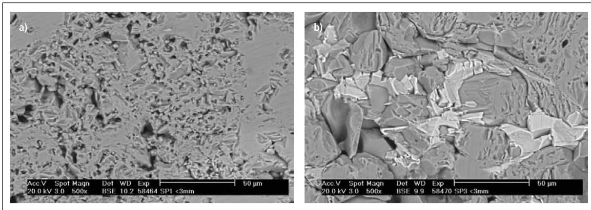
**Fig. 2a–b** BSE images of sintered samples from AR 78 <3 mm without Al<sub>2</sub>TiO<sub>5</sub> (a), and with 12 mass-% Al<sub>2</sub>TiO<sub>5</sub> (b)
