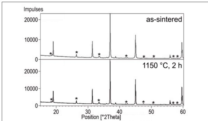
**Fig. 8** X-ray diffractograms of MA spinel ceramic from raw material <math><20\ \mu\text{m}</math> with 12 mass-%  $\text{Al}_2\text{TiO}_5$  after sintering and after subjecting a test specimen in the RFDA apparatus to a temperature of 1150 °C (see Fig. 7 b); \* $\text{Al}_2\text{TiO}_5$
