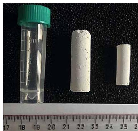
**Fig. 3** Photograph of a mold (l.), a sample after withdrawal from the desiccator (middle), and a sample after sintering at 1650 °C for 3 h (r.); all samples prepared with both alumina and mullite particles
