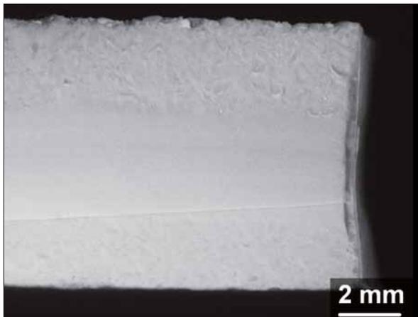
**Fig. 3** Side view of an eleven-layer laminate with the layer sequence A6-3\*A4-3\*A2-3\*A4-A6
