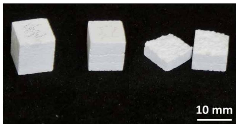
**Fig. 9** Three-layer alumina laminates (A5) after fourfold downward thermal shock ( $\Delta T = 1000$  °C, quenching in water): no visible damage (l.), partially delaminated sample (middle), completely delaminated laminate (r.)
