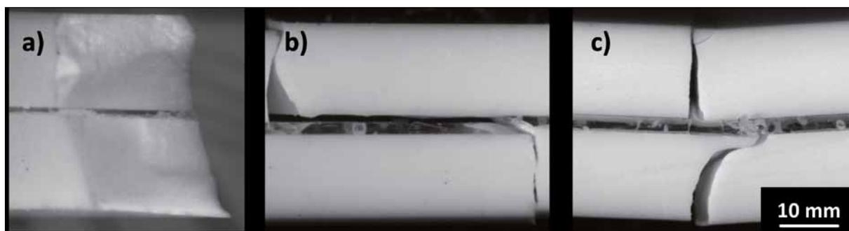
**Fig. 7a–c** Optical microscope images of fractured surfaces of ceramic-glass laminates after four-point bending test at: a) room temperature, b) 600 °C, and c) 700 °C
