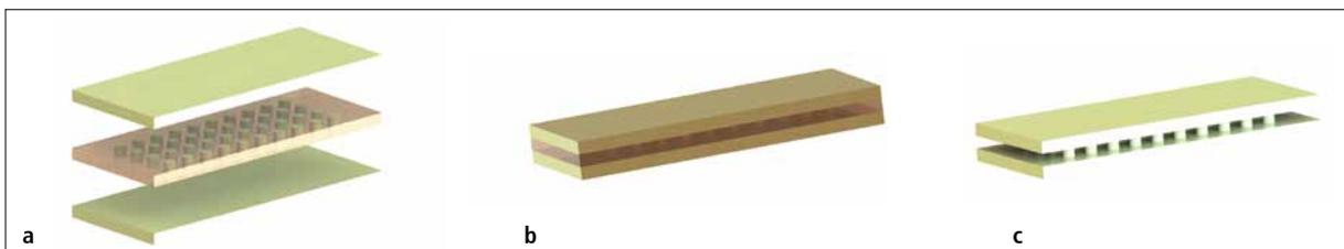
**Fig. 3a–c** Pattern of pure binder tape with filled vias between two green tapes (a), pattern of laminated multilayer with pure binder tape in between (b), and pattern of sintered multilayer after removing of organics (c)
