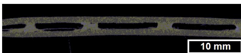
Fig. 12 CT-image of CaAl-multilayer manufactured with pure binder tape inside
