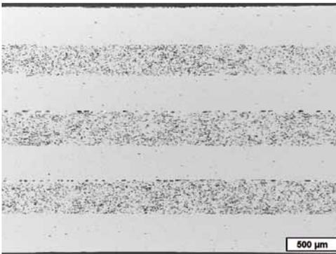
**Fig. 1** SEM-image of cross-section of MgO-ZrO<sub>2</sub>-multilayer with non-linear graded microstructure (0%/25%.../25%/0% porosity) manufactured by multilayer technology
