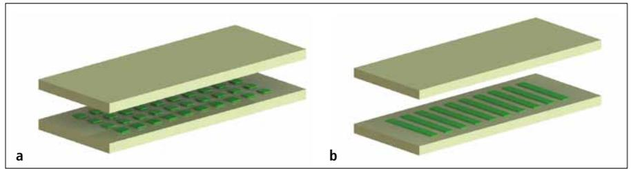
**Fig. 2a–b** Selective lamination by dot-shaped deposition of joining suspension (a), and selective lamination by deposition of joining suspension in different lines (b)
