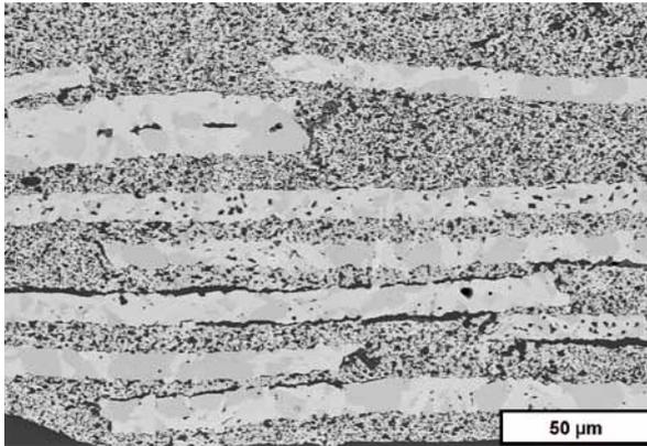
**Fig. 6** SEM-image of cross-section of CaAl-multilayer with CaAl-platelets
