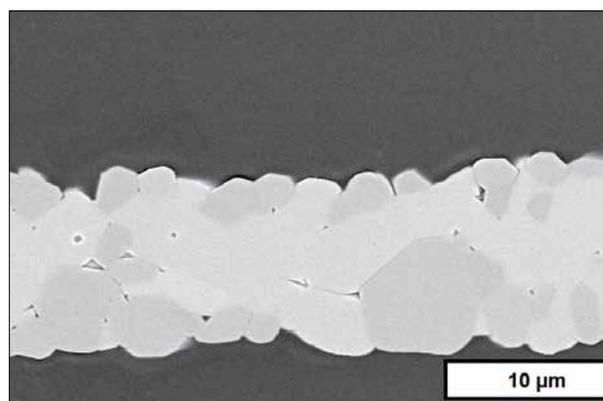
**Fig. 5** SEM-image of cross-section of a single CaAl-platelet
