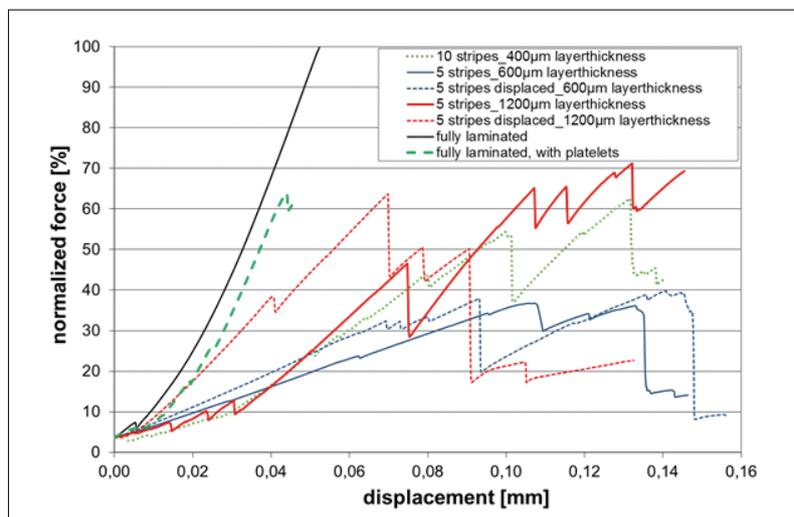
Fig. 11 Generic curves as results of 4-point-bending-tests for different CaAl-multilayers
