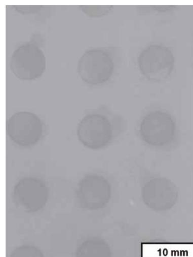
Fig. 13 Radiography-image of CaAl-multilayer manufactured with pure binder tape inside
