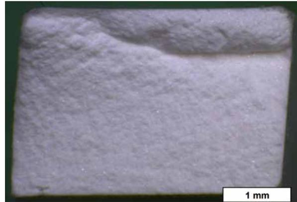
**Fig. 7** Fracture surface of homogeneous CaAl-multilayer
