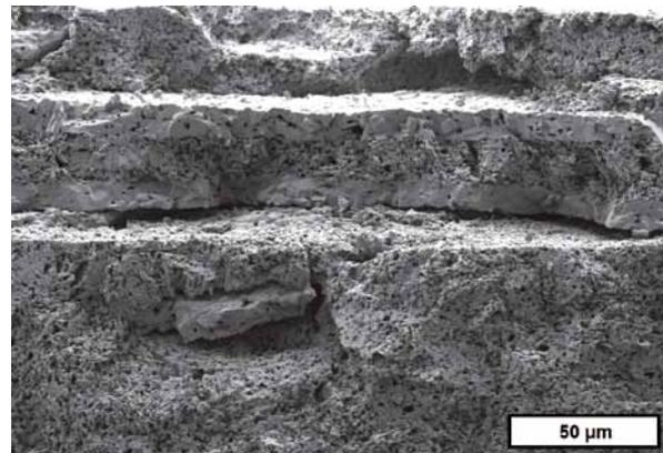
**Fig. 9** SEM-image of fracture surface of CaAl-multilayer with CaAl-platelets
