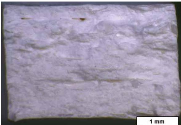
**Fig. 8** Fracture surface of CaAl-multilayer with CaAl-platelets
