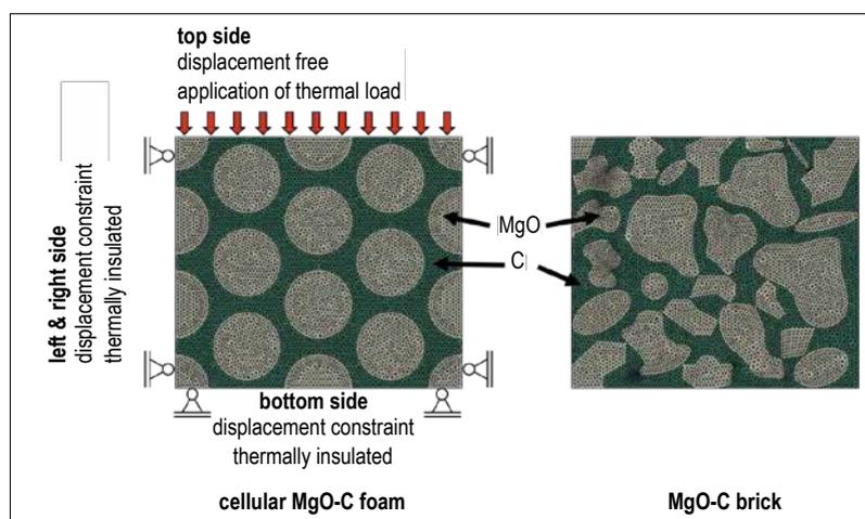
**Fig. 2** RVE microstructure of the MgO–C foam including the applied boundary conditions (l.), and the RVE microstructure of the common MgO–C brick (r.)
