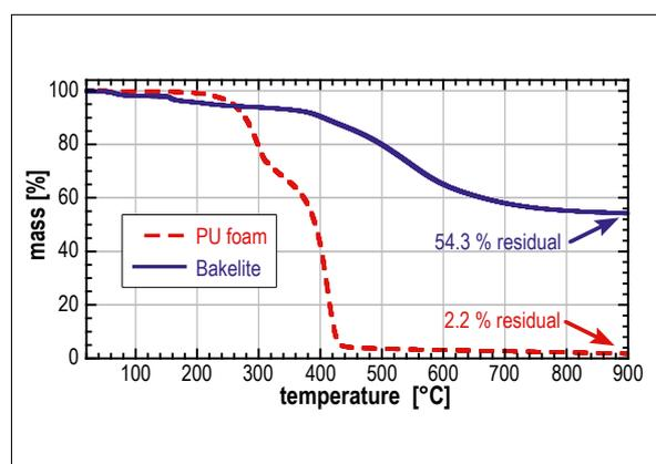
**Fig. 3** Thermogravimetric analysis of the polyurethane foam and the Bakelite resin
