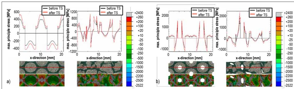
**Fig. 13** a) Stress distribution in the microstructure of a MgO-C foam (l.), and of a MgO-C brick (r.) before and after Thermal Shock (TS): maximal principal stress (top), microstructure (middle) and contour plot after thermal shock (bottom); b) same for MgO-C containing air-filled pores
