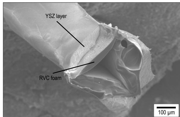
Fig. 7 SEM image of a reticulated vitreous carbon foam coated with yttrium-stabilized zirconia (green body)
