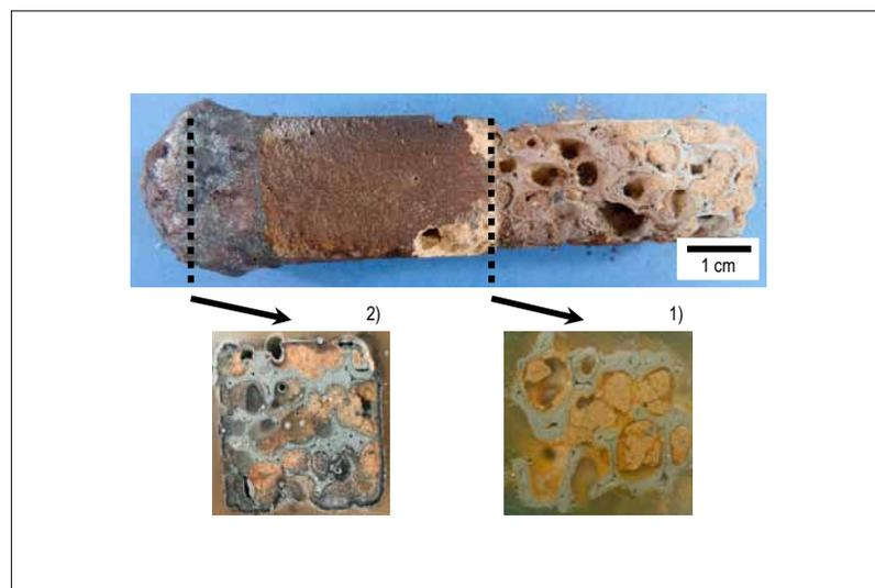
**Fig. 11** Cross sections of the MgO–SiC laboratory sample after the corrosion testing; the bar was fixed on the right side
