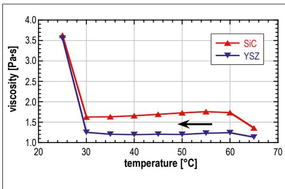
Fig. 6 Viscosities of antioxidant slurries containing carrageen as gelling additive
