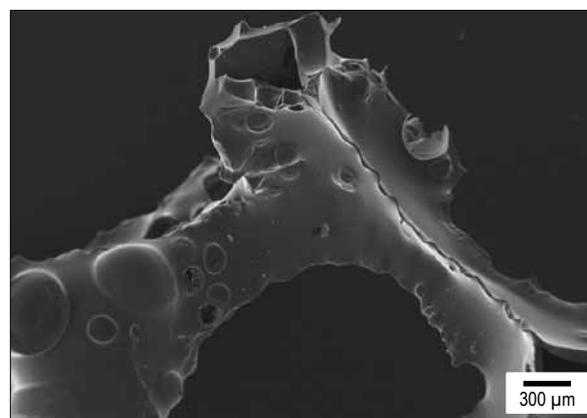
**Fig. 4** SEM image of a strut of RVC foam pyrolyzed at 1000 °C
