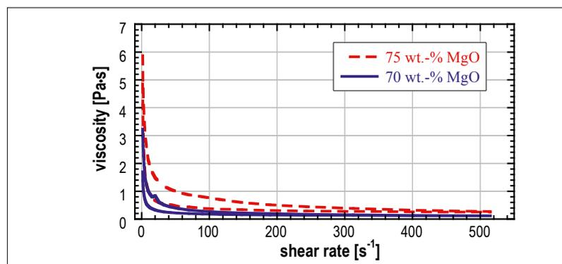
**Fig. 9** Rheological behaviour of MgO slurries with different solid content
