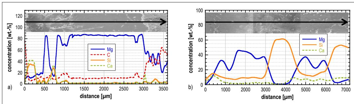
**Fig. 12** a) Line scan of the reference sample (section 2) in Fig. 10; b) Line scan of the laboratory MgO-SiC sample (section 2) in Fig. 11
