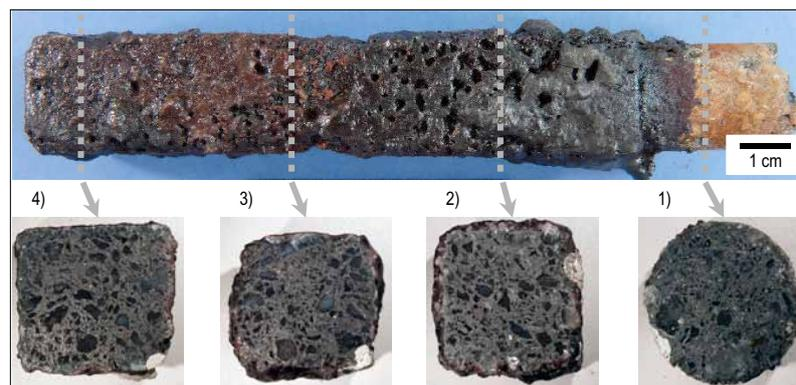
**Fig. 10** Cross sections of the reference sample after the corrosion testing; the bar was fixed on the right side
