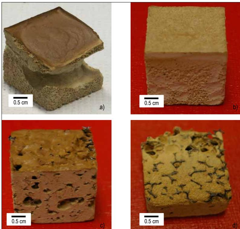
Fig. 8a–d Development steps passed during casting of MgO slurries: a) shrinkage during drying; b) optimized layer by layer casting; c) pores after infiltration into the PU foam; and d) improvement by additional shaking
