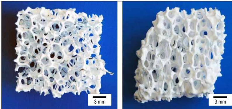
Fig. 5 Two examples for RVC foams coated with YSZ (green body)
