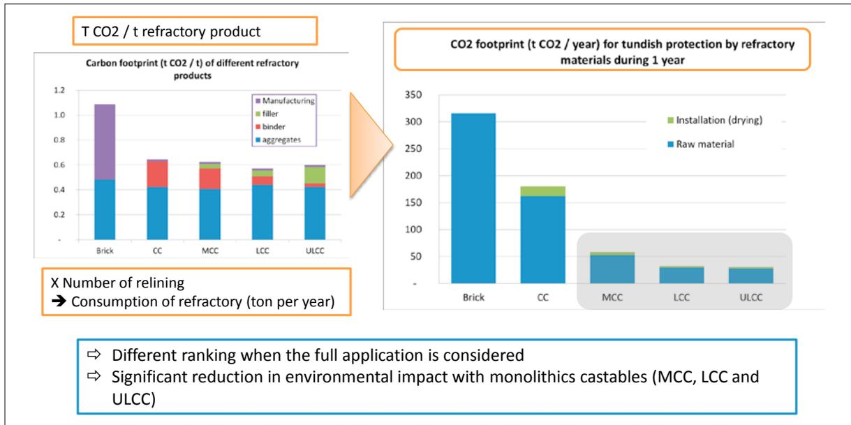
**Fig. 5 From CO<sub>2</sub> footprint for 1 t of refractory product to impact of full application (1 year of tundish protection with permanent lining)**
