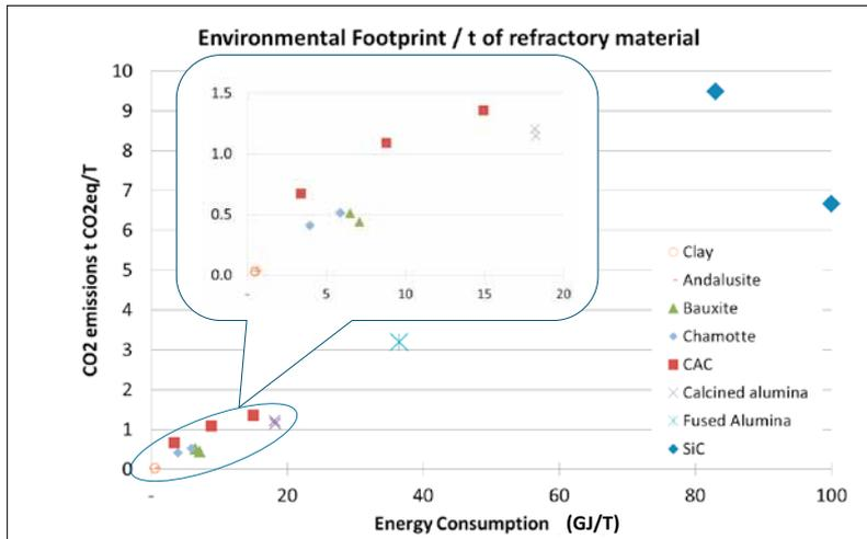
**Fig. 4** Environmental footprint for 1 t of refractory material
