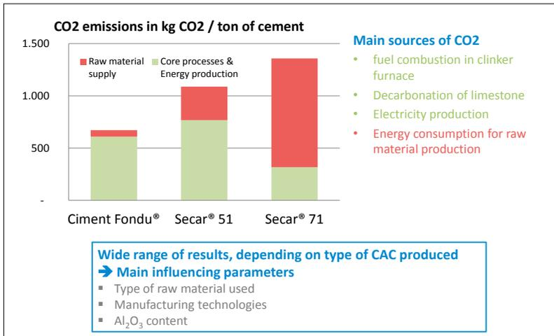
**Fig. 3** Impact of raw material production: example of CO<sub>2</sub> emissions of CAC production [kg CO<sub>2</sub>/t]
