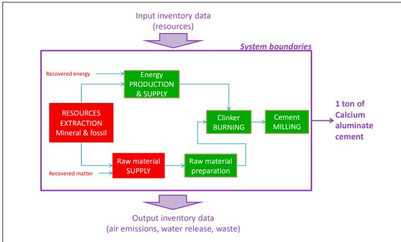
**Fig. 2** System boundaries of calcium aluminate cement production, from cradle to gate
