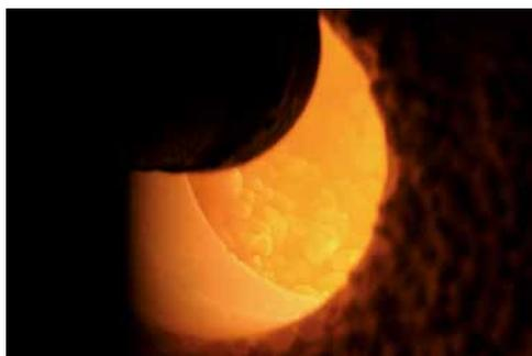
**Fig. 2** View into the dynamic laboratory rotary drum furnace at 1450 °C with clinker nodules inside
