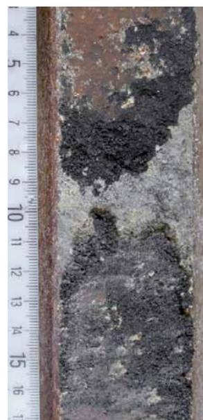
**Fig. 4 Surface of a magnesia-spinel refractory sample after testing at 1450 °C (scale in cm); adhering clinker (black) formed a coating layer**
