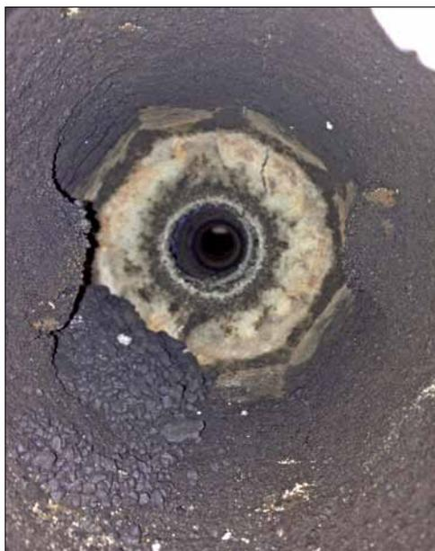
**Fig. 3** Laboratory rotary drum furnace after 8 charges of raw mix had been fired to clinker
