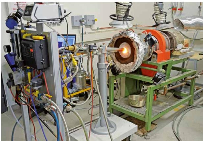
**Fig. 1** Dynamic laboratory rotary drum furnace
