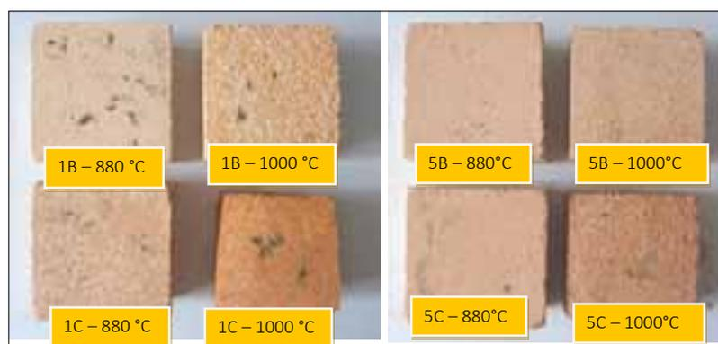
**Fig. 7 Samples after firing – clay B and clay C**
