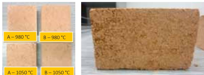
**Fig. 6 Samples A and B after firing**
