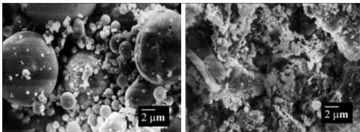
**Fig. 1** Morphology of grains in class F fly ash (l.), and class C fly ash (r.)
