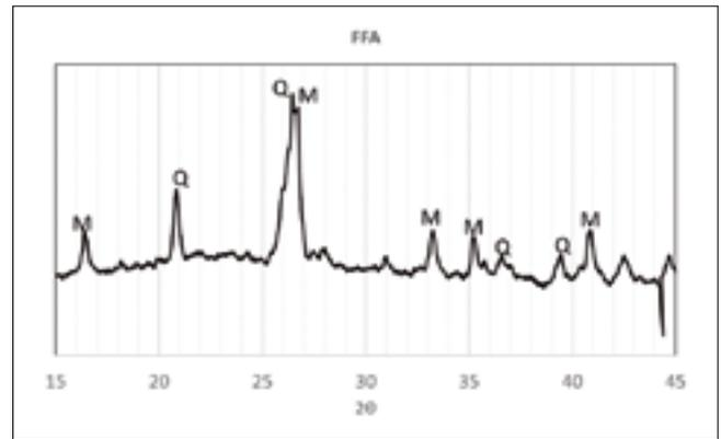
Fig. 3 X-ray analysis – class F fly ash (Q-quartz; M-mullite)
