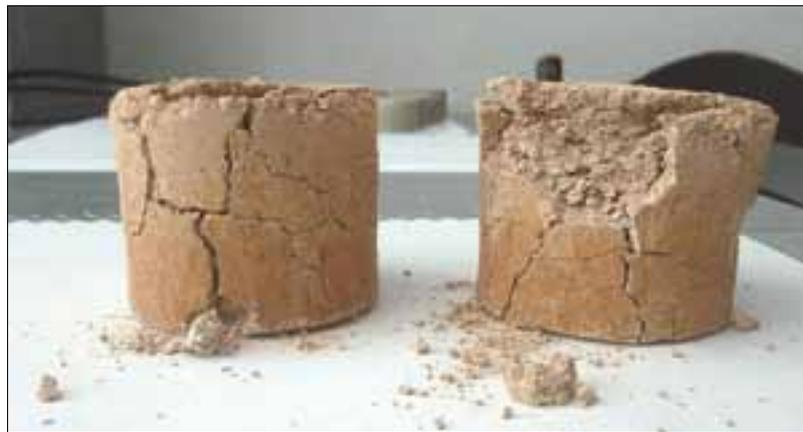
**Fig. 8 Cracks and additional volume changes after firing**
