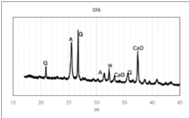
Fig. 2 X-ray analysis – class C fly ash (Q-quartz; A-anhydrite; H-hematite)
