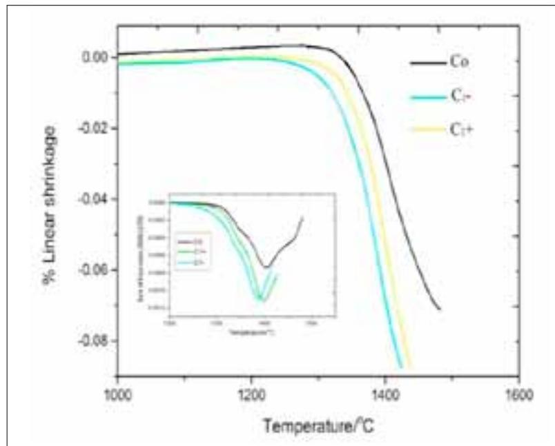
**Fig. 6** Comparison of TMA patterns  $C_0$ ,  $C_{1+}$  and  $C_{1-}$  matrices respectively: linear shrinkage vs. temperature plot with the inset rate of expansion vs. temperature
