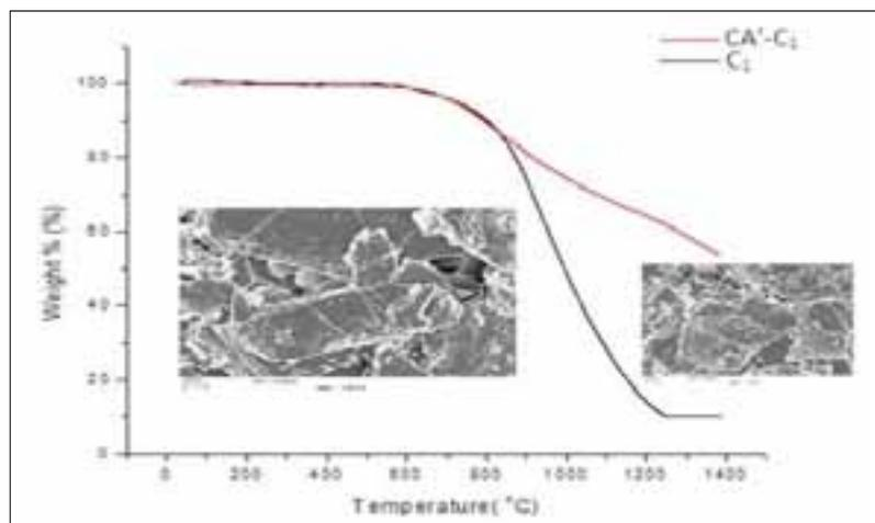
**Fig. 1** Comparison of TGA patterns of coated and uncoated graphites with their inset SEM micrographs (LHS: C<sub>1</sub>; RHS: CA'-C<sub>1</sub>)
