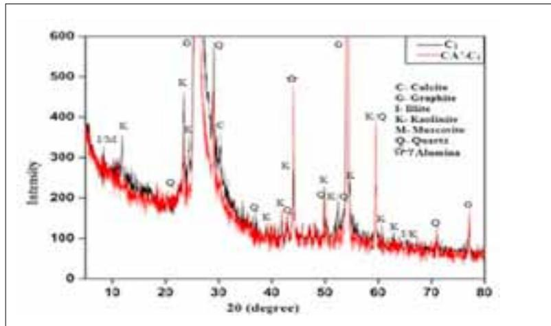
Fig. 2 Combined XRD plots of coated and uncoated graphites
