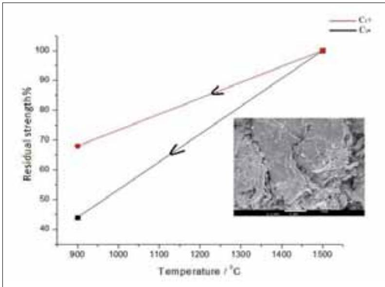
**Fig. 4** Comparison of thermal shock resistance of  $C_{1+}$  and  $C_{1-}$  castables respectively with the inset SEM micrograph of the 1500 °C fired  $C_{1+}$  sample
