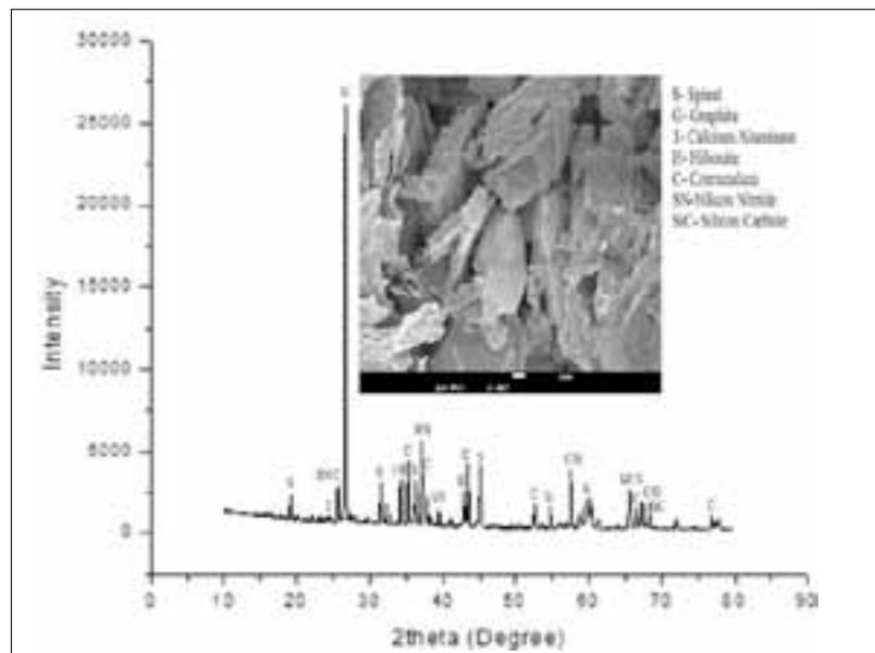
**Fig. 7** XRD plot of the  $C_{1+}$  matrix fired at 1500 °C with inset SEM micrograph
