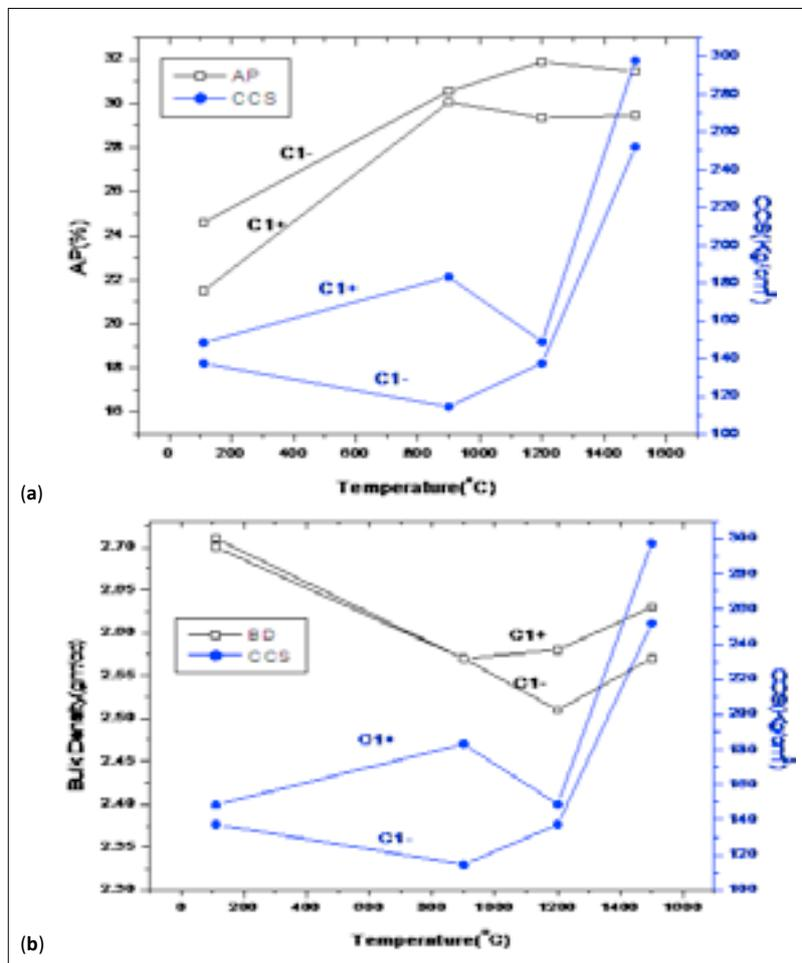
Fig. 3 Comparison of variation in physical properties of C<sub>1+</sub> and C<sub>1-</sub> castables respectively with increasing temperatures: (a) AP vs. CCS plot, (b) BD vs. CCS plot
