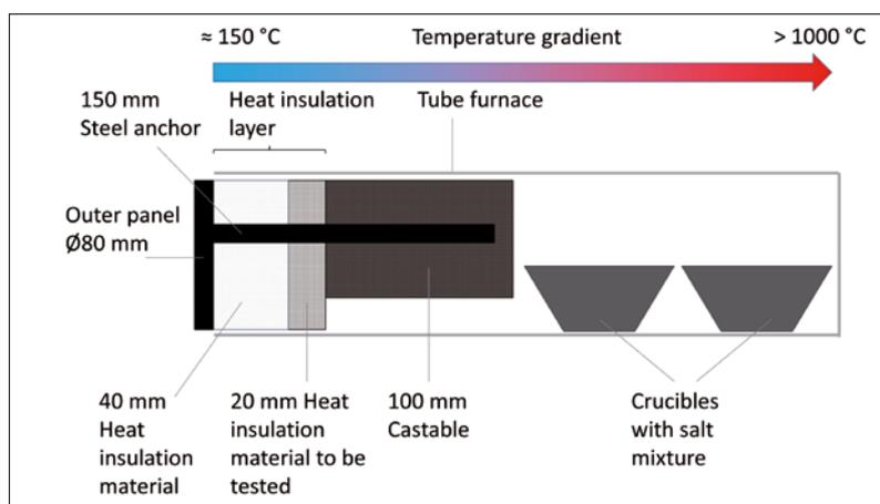
Fig. 2 Schematic draft of the laboratory testing facility according to Schlegel [9]
