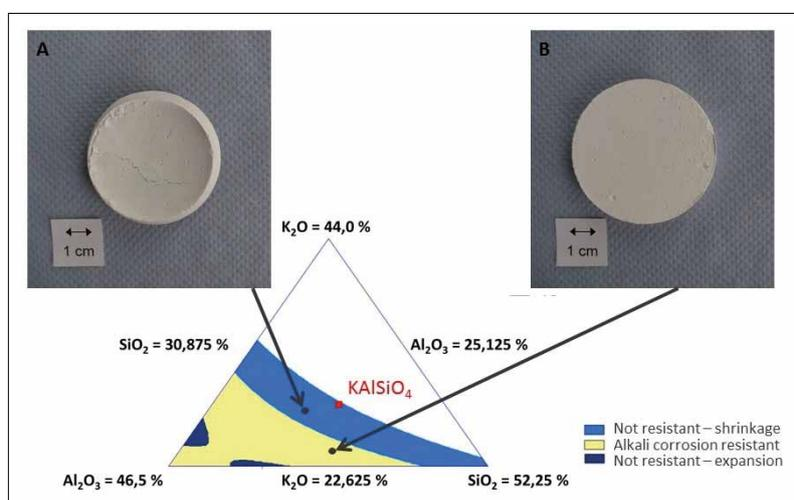
Fig. 3 Compositional regions in the system  $K_2O-Al_2O_3-SiO_2$  (compositions in mass-%) with prediction of their alkali corrosion resistance identified by regression models with two exemplary points A and B, after [12, 13]
