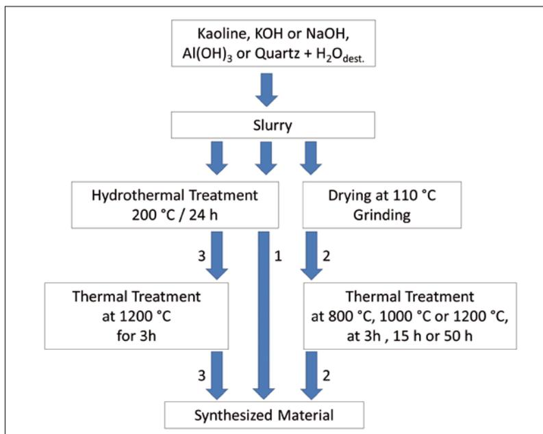
**Fig. 1 Schematic representation of the investigated synthesizing routines: 1 – hydrothermal routine, 2 – thermal routine, 3 – combined routine (after [9])**
