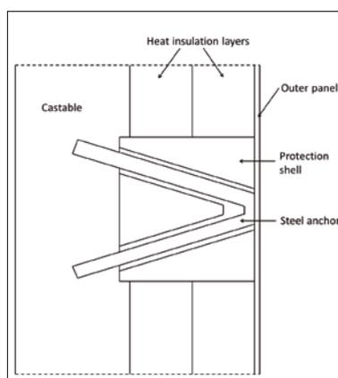
**Fig. 4** Schematic draft of the protection shells for steel anchors, after [10]
