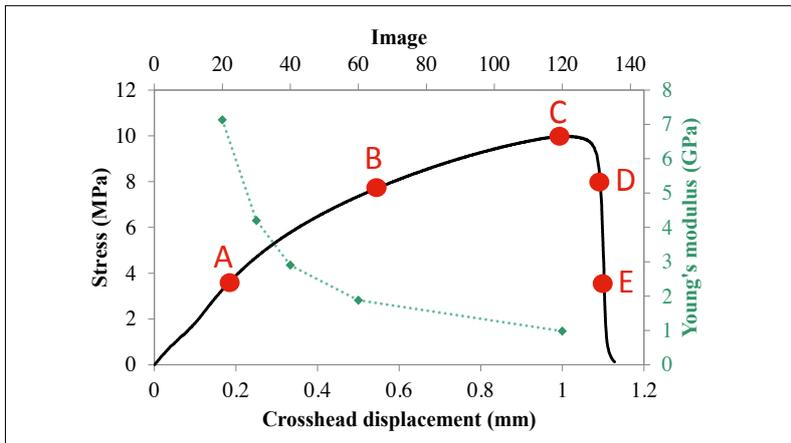
**Fig. 1** Experimental stress-displacement curve and evolution of Young's modulus of AT VF obtained by FEMU-U
