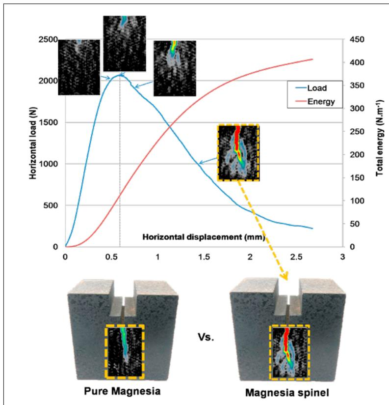
**Fig. 4** Horizontal load-displacement and energetic curves for the MSp sample; the strain maps obtained along X-axis are represented in different steps during the wedge splitting test
