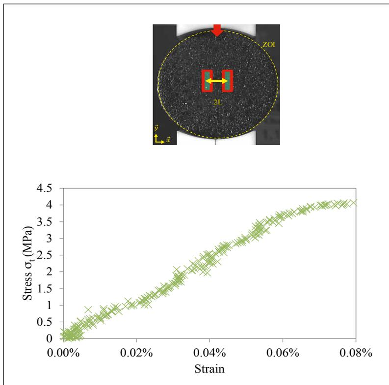
**Fig. 5** Stress-strain curve obtained using DIC during a Brazilian test
