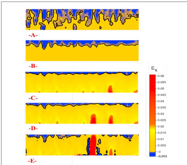
**Fig. 2** Maps of strains along X-axis for the five times defined in the stress-displacement curve (a)
