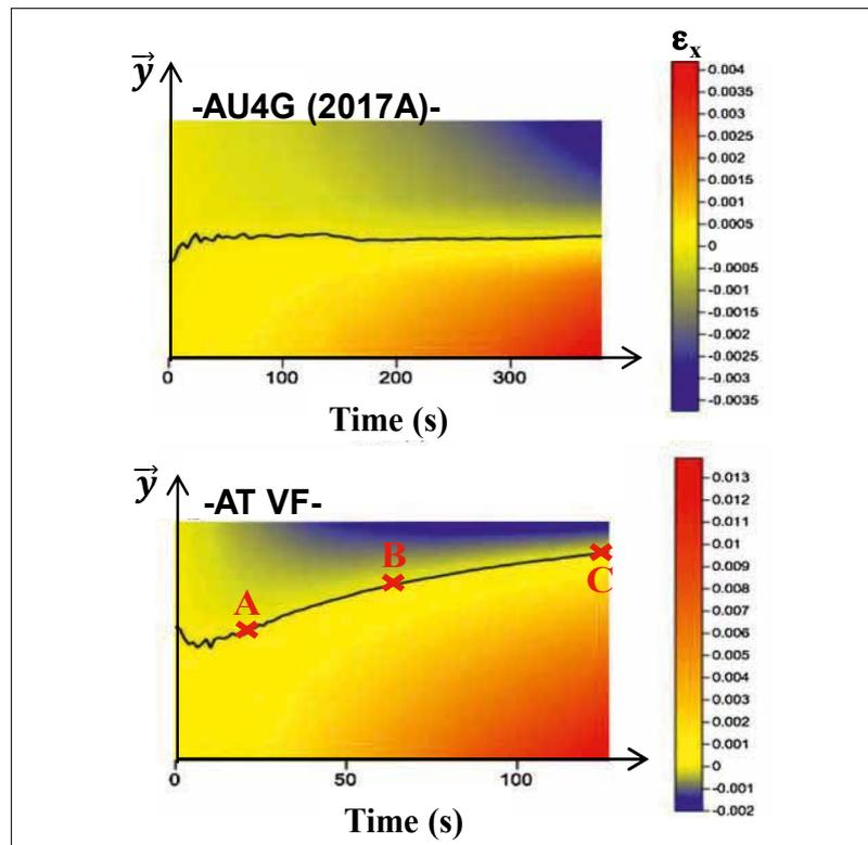
**Fig. 3** Evolution of strain fields during the test for an aluminium sample (a), and AT VF sample (b)
