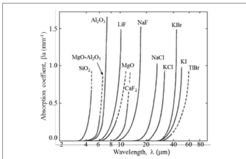
Fig. 3 Absorption coefficient as a function of wavelength for ceramic materials [3]
