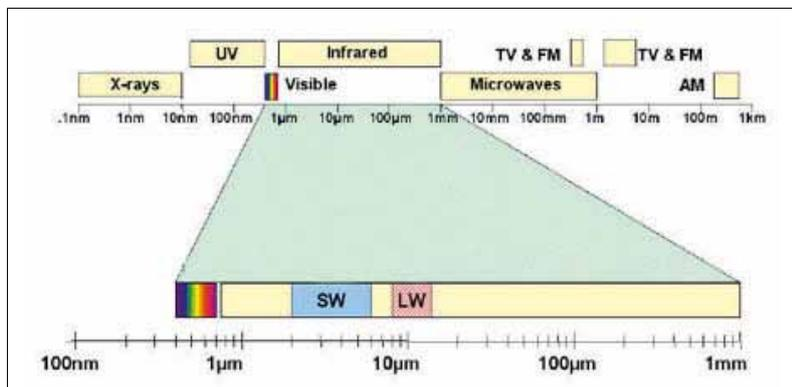
**Fig. 1** Electromagnetic spectrum of energy highlighting infrared radiation, where the shortwave (SW) corresponds to a range of 3–5  $\mu\text{m}$  and longwave (LW) to 8–12  $\mu\text{m}$  [2]
