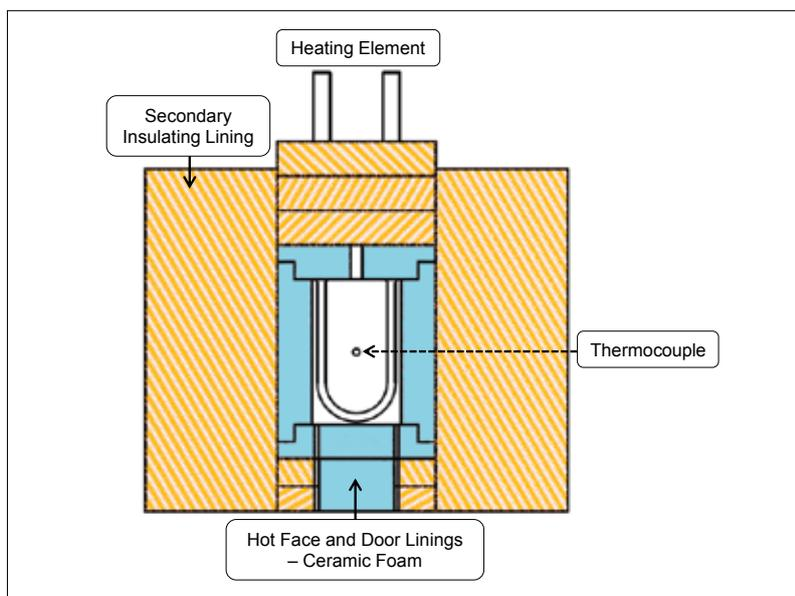
**Fig. 4** Schematic drawing of the glass melting furnace for 1700 °C
