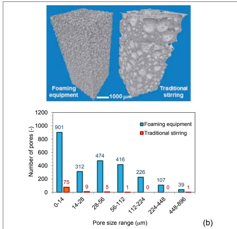
**Fig. 6 a–b** μCT images of  $Al_2O_3$  foams after sintering at 1500 °C for 5 h produced by (a) foaming equipment (P: 76 vol.-%) or traditional stirring (P: 60 vol.-%), and (b) the volumetric pore size distribution for both processing routes
