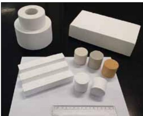
**Fig. 5** Al<sub>2</sub>O<sub>3</sub>-based foam pieces produced by direct-foaming equipment [6]
