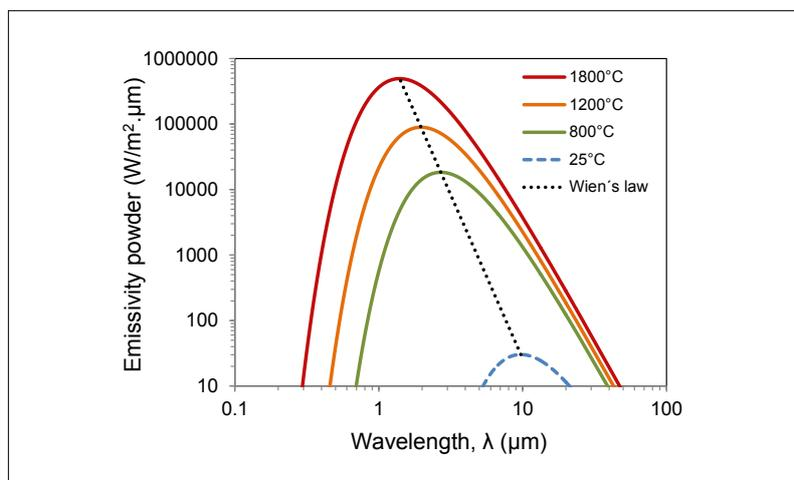
Fig. 2 Emissivity power as a function of wavelength and temperature [3]
