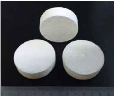
**Fig. 8** Foamed ceramic samples after 10 cycles of thermal shock testing at 1700 °C in air
