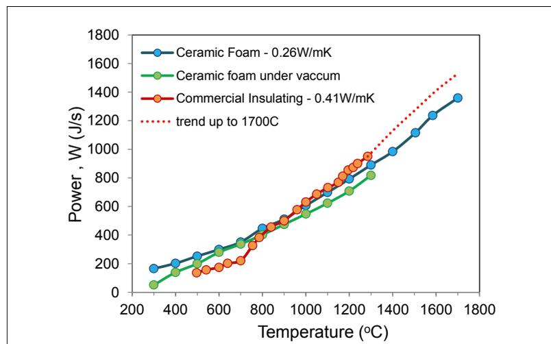
**Fig. 7** Power supplied to the heating elements as a function of temperature for two types of insulating material lining
