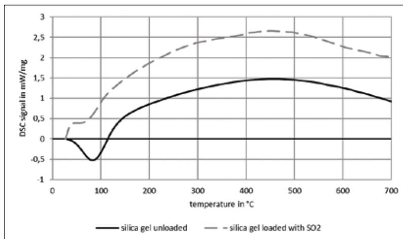
Fig. 8 Differential scanning calorimetric measurement of unloaded silica gel and silica gel loaded
