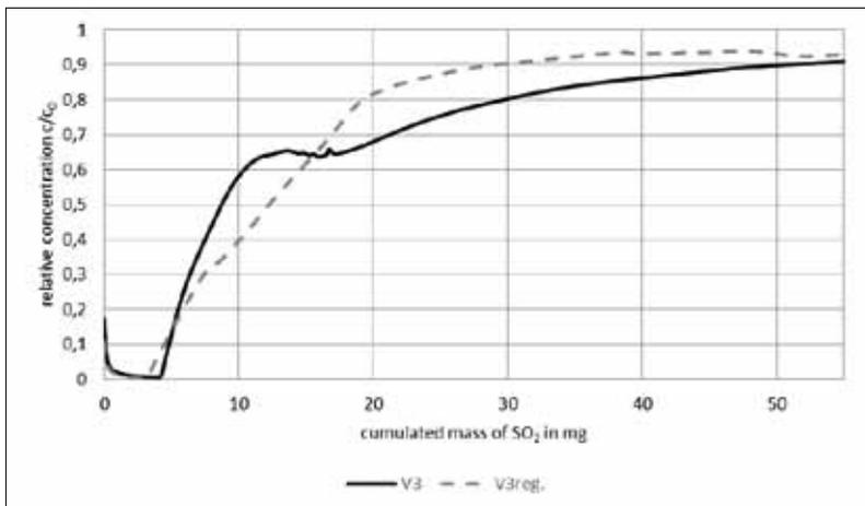
**Fig. 11** First (V3) and second  $SO_2$  adsorption (V3<sub>reg.</sub> after regeneration), 70 % relative humidity
