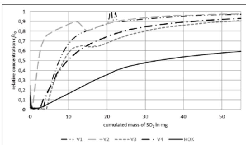
Fig. 3  $\text{SO}_2$  concentration of silica gels V1–V4 and HOK over time
