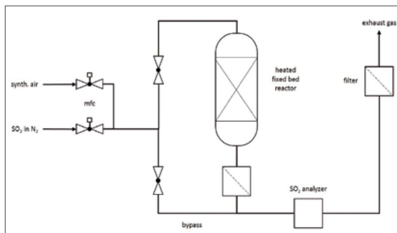
**Fig. 1** Experimental set up of SO<sub>2</sub> breakthrough curve measurements
