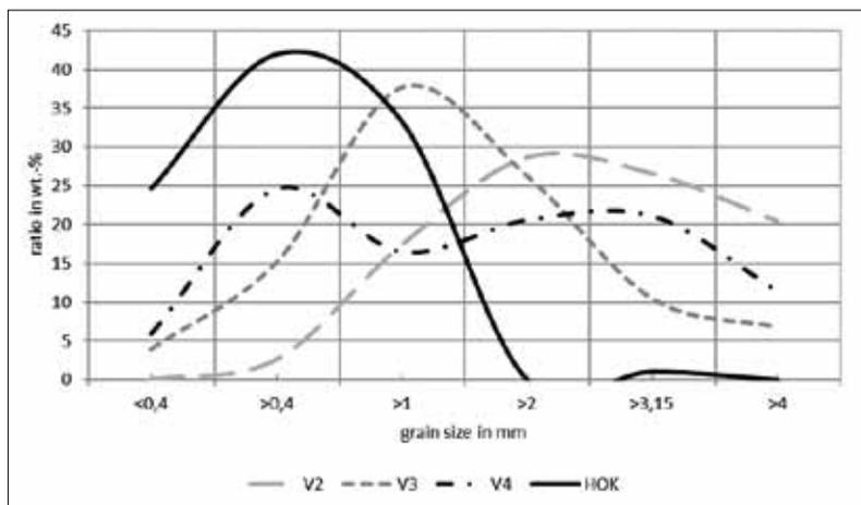
Fig. 2 Grain size distribution of different silica gels and HOK medium
