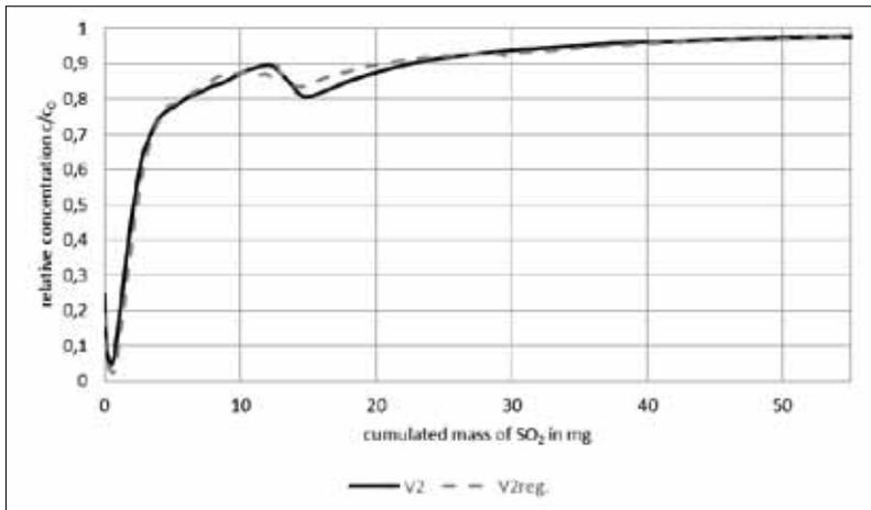
**Fig. 10** First (V2) and second  $SO_2$  adsorption (V2<sub>reg.</sub> after regeneration), 45 % relative humidity
