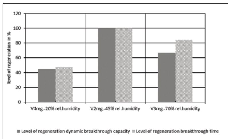
**Fig. 14** Level of regeneration of the breakthrough time and dynamic breakthrough capacity of silica gels V2<sub>reg.</sub>, V3<sub>reg.</sub> and V4<sub>reg.</sub>
