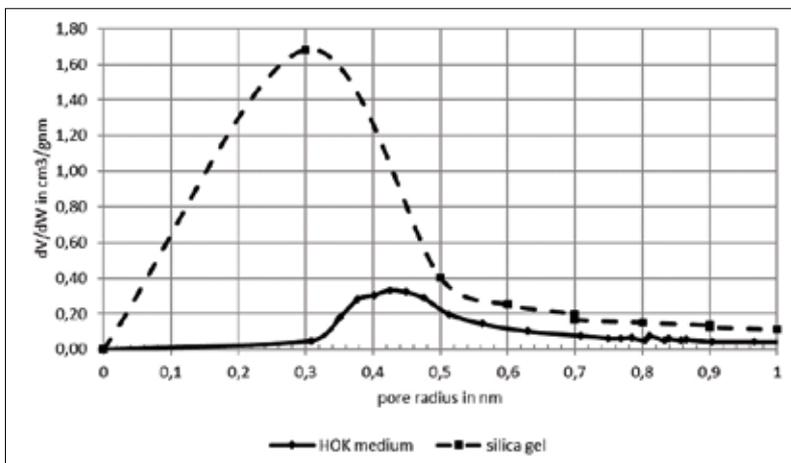
**Fig. 5** Pore size distribution by nitrogen adsorption measurements of HOK medium and silica gel
