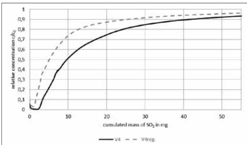
**Fig. 12** First (V4) and second  $SO_2$  adsorption (V4<sub>reg.</sub> after regeneration), 20 % relative humidity
