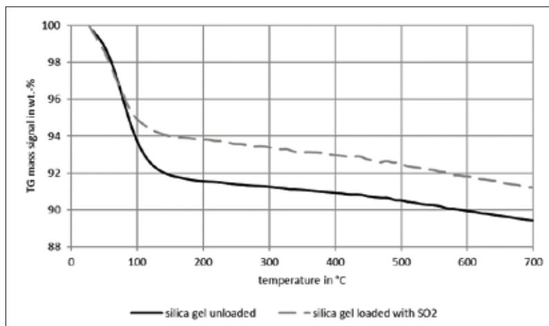
Fig. 9 Thermogravimetric measurement of unloaded silica gel and loaded silica gel
