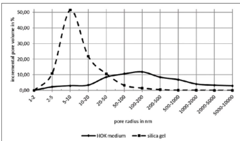
**Fig. 6** Pore size distribution by mercury intrusion measurements of HOK medium and silica gel
