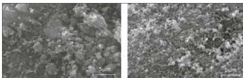
Fig. 7 Scanning electron microscopic images of A) HOK medium, and B) silica gel
