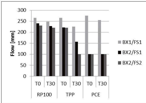
Fig. 3 Initial vibration flow and after 30 min
