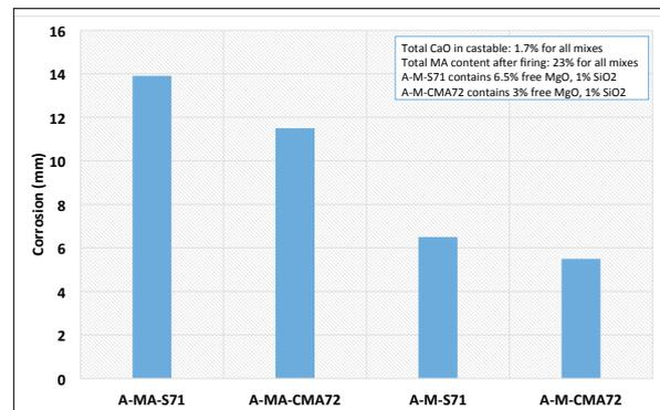
Fig. 11 Corrosion of A-MA and A-M castables
