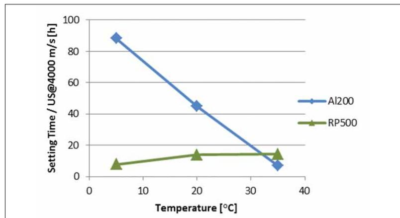
Fig. 5 Time to reach an ultrasound speed of 4000 m/s
