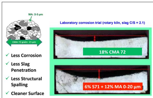
Fig. 10 Samples after rotary slag corrosion test
