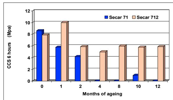
Fig. 9 Early strength development as function of dry-mix storage time
