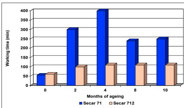
Fig. 8 Working time as function of dry-mix storage time
