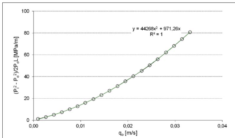
Fig. 3 Darcy plot: measurements performed on refractory B; the parabolic shape indicates that inertial effects arose
