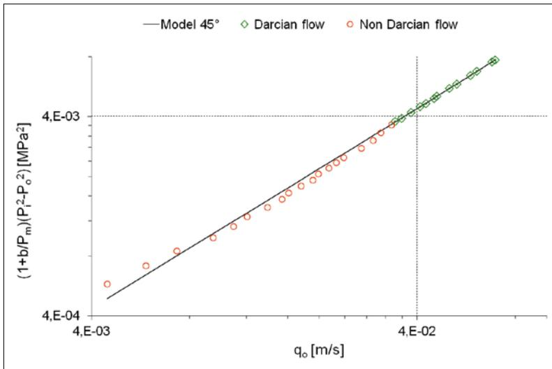
**Fig. 1** Corrected Darcy plot of refractory A according to Dranchuk [14]
