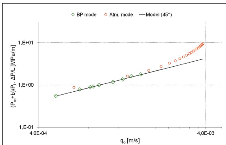
Fig. 4 Corrected Darcy plot of refractory B according to Dranchuk [14]: the straight line with its slope equal to 1 shows that any measurements in atmospheric mode was obtained in Darcy flow regime conditions (circles), all the points obtained in backpressure mode (diamonds) fulfilled the conditions
