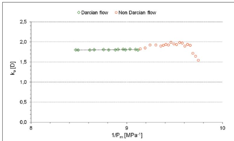
Fig. 2 Klinkenberg plot: determination of intrinsic permeability using measurements performed in Darcy flow regime conditions on refractory A
