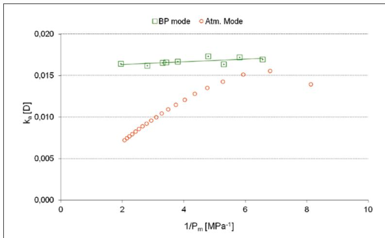
**Fig. 5** Klinkenberg plot of refractory B: intrinsic permeability is derived from measurements performed in backpressure mode
