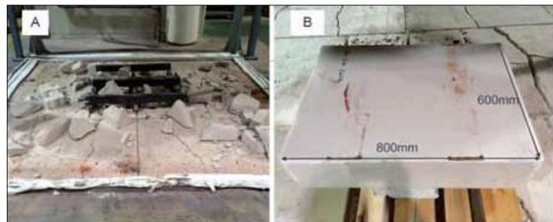
**Fig. 7** 300 kg blocks after rapid heat-up: A) drying schedule-A, and B) drying schedule-B6
