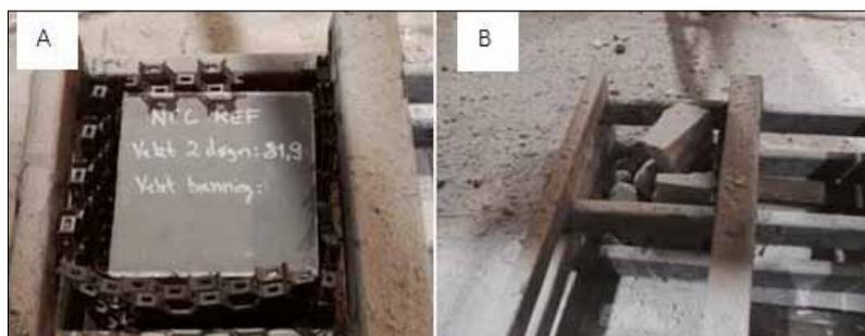
**Fig. 9** ~80 kg block before (A), and after (B) explosion resistance test
