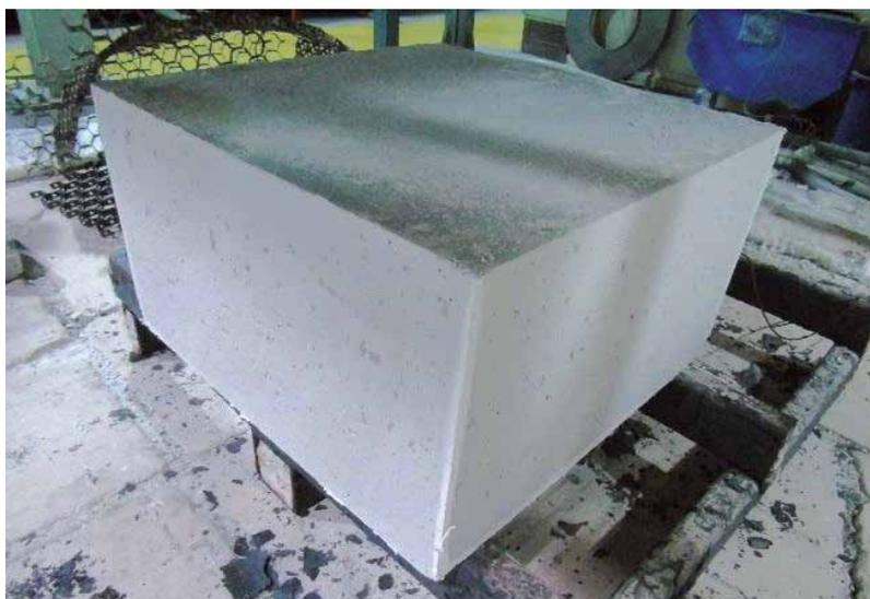
**Fig. 12** ~400 kg block with EMSIL-DRY after explosion testing at 850 °C
