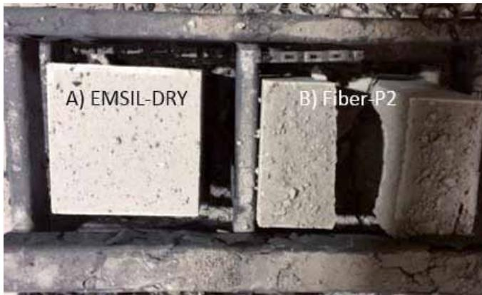
**Fig. 10** ~75 kg blocks after explosion resistance test: A) 0,1% EMSIL-DRY™, and B) 0,1% Fiber-P2
