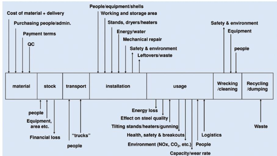
**Fig. 1** Different aspects in the refractory lifecycle of the steel ladle influencing the Value-in-Use
