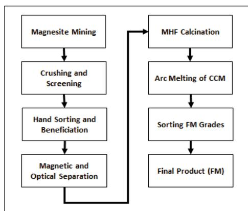
Fig. 1 Flow diagram of fused magnesia production
