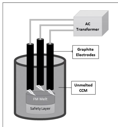
**Fig. 2** Electric arc furnace for production of fused magnesia
