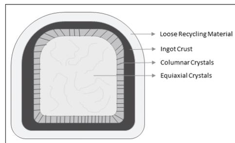
**Fig. 3** Zonal structure of fused MgO ingot
