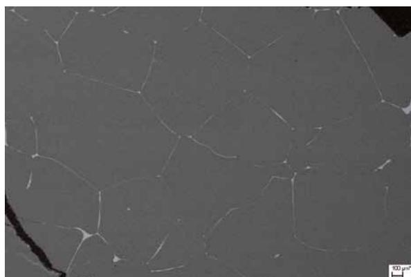
**Fig. 5** SEM image of A1 sample
