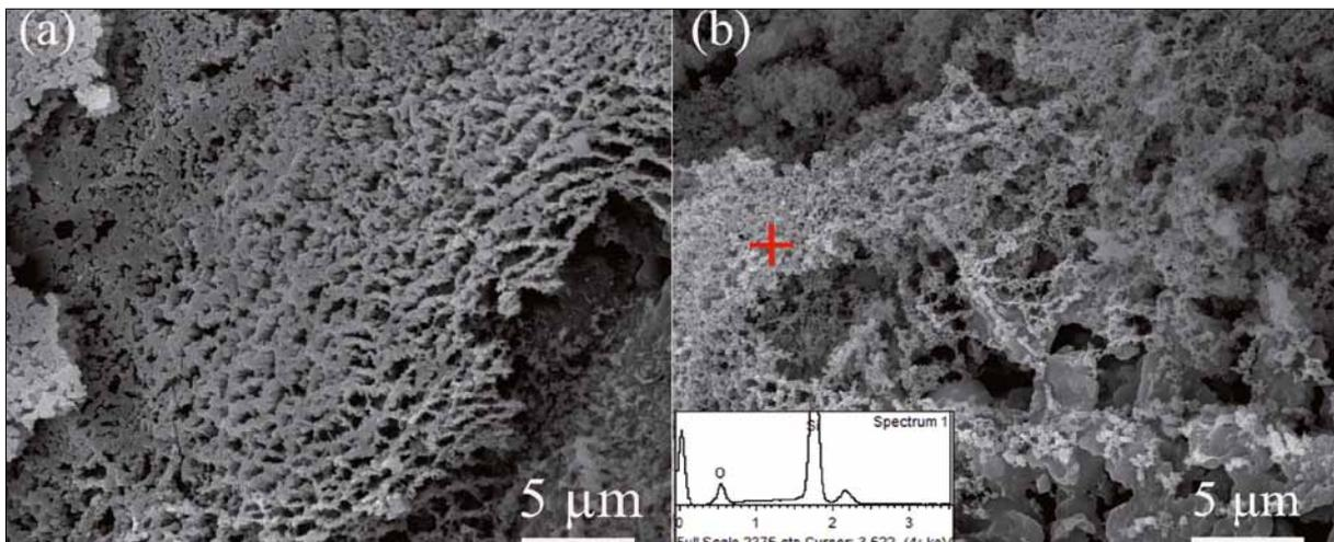
Fig. 11 a–b SEM photograph showing the further reaction occurs in residual graphite in sample SNC-g after 9 quenching cycles
