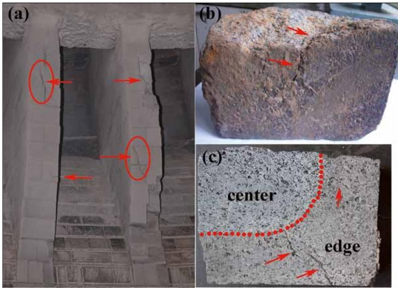
**Fig. 1 a–c** (a)  $\text{Si}_3\text{N}_4$ -reaction-bonded SiC-bricks applied in ramp area of dry coke quenching furnaces after 18 months; the spalling phenomenon and cracks was found in bricks; (b) cracks were formed in brick edge after 36 months; (c) the cross section morphology of brick shown in (b) [9]
