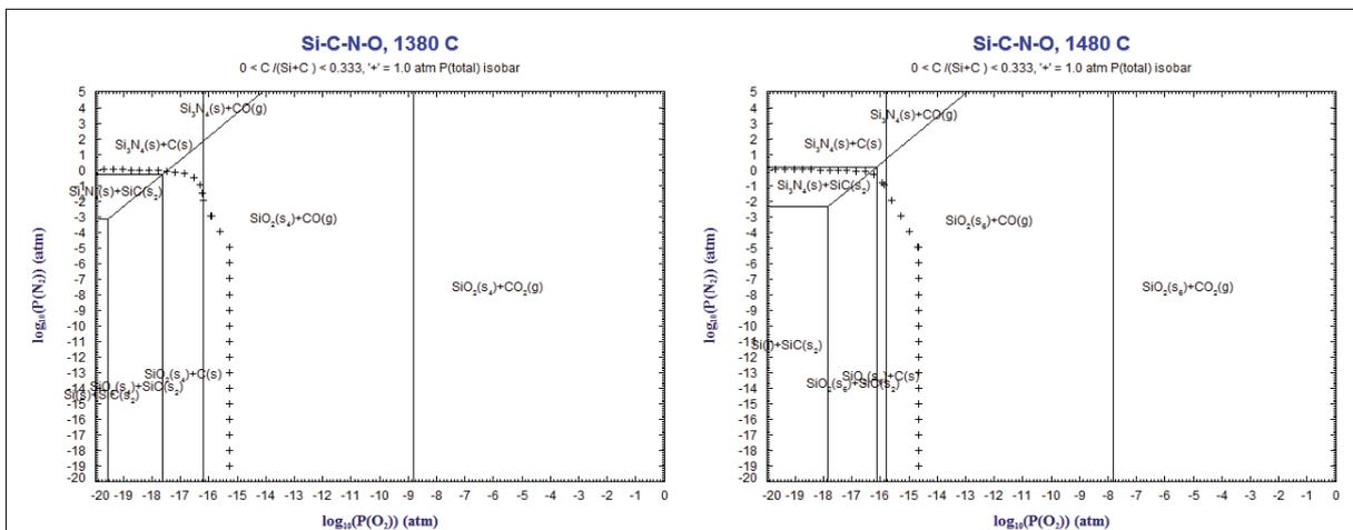
**Fig. 5** Si–C–N–O predominance area diagrams at 1380 °C and 1480 °C
