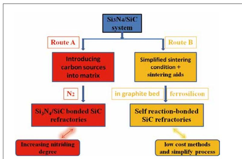
Fig. 3 Schematic of the two processing routes studied here
