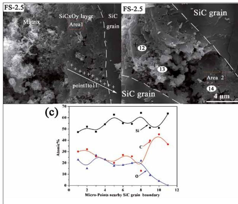
**Fig. 16 a–c** SEM micrographs of a fracture surface in sample FS2,5, showing the bonded morphology of SiC grain/matrix (a, b); energy spectrum analysis of micro-points nearby SiC grain boundary (c) [22]
