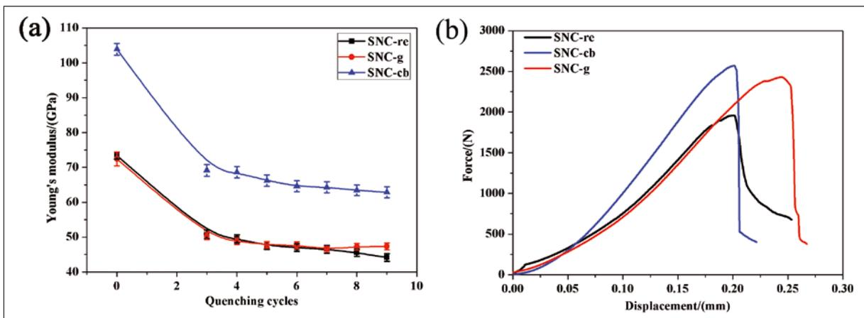
Fig. 10 a–b Evolution of Young’s modulus as a function of quenching cycle (samples tested with 1100–20 °C) (a), and force-displacement curves of samples after 9 quenching cycles with samples sizes of 25 mm × 30 mm × 140 mm (b) [23]
