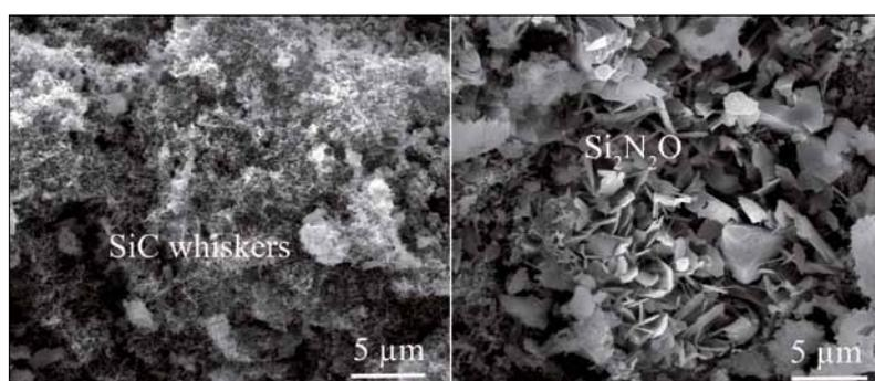
**Fig. 13** SEM images of samples matrix, showing that SiC whiskers and plate-like  $\text{Si}_2\text{N}_2\text{O}$  formed in the matrix of samples FS-2,5
