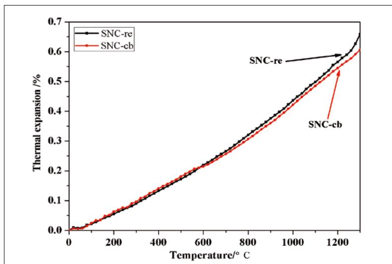
**Fig. 12** The thermal expansion of samples as a function of temperature from 20–1300 °C [23]
