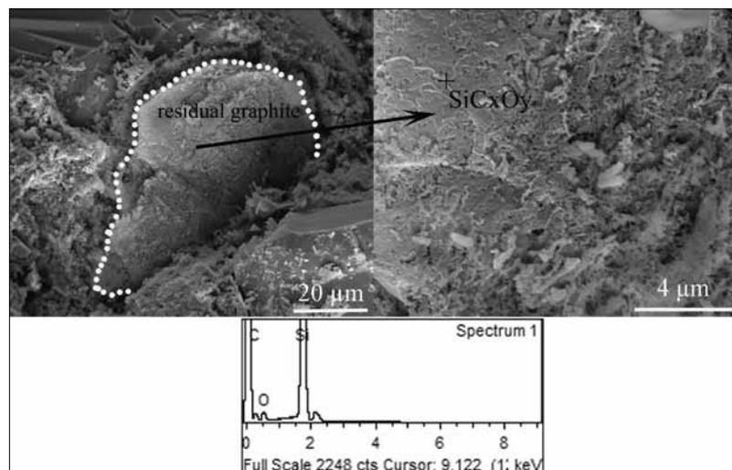
**Fig. 8 a–b** The bonded morphology in sample SCN-g interior: a) residual graphite existed between SiC aggregate and matrix, and b) SiC<sub>x</sub>O<sub>y</sub> formed on the residual graphite surface (SEI) [23]
