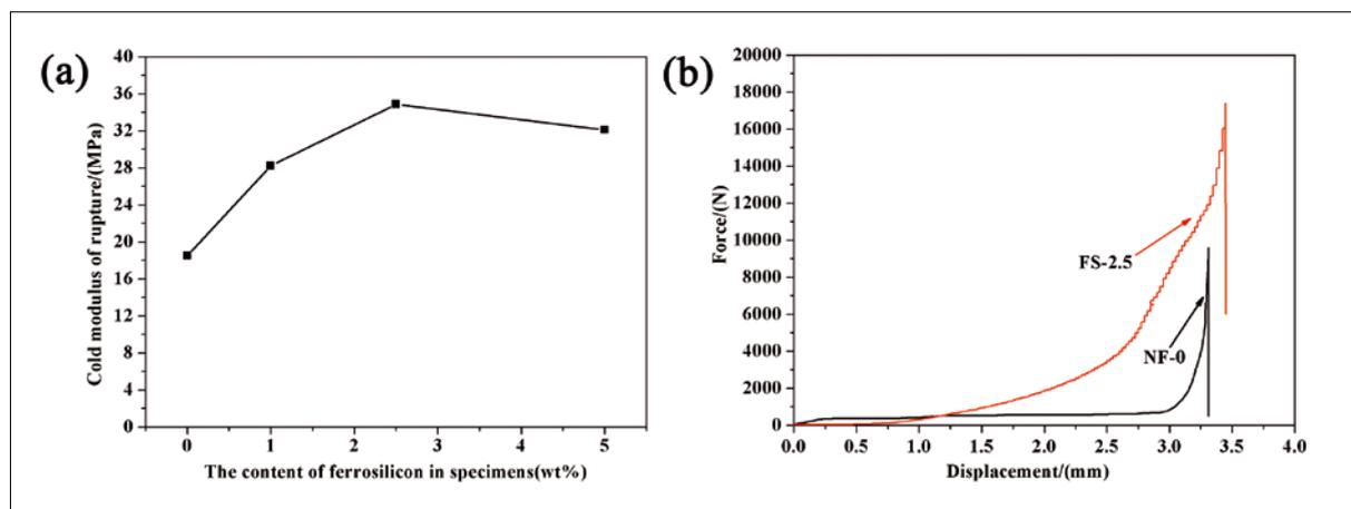
**Fig. 17 a–b** CMOR of samples containing different ferrosilicon content after firing (a), and force-displacement curves of samples containing 2,5 mass % and without ferrosilicon after firing (b) [22]
