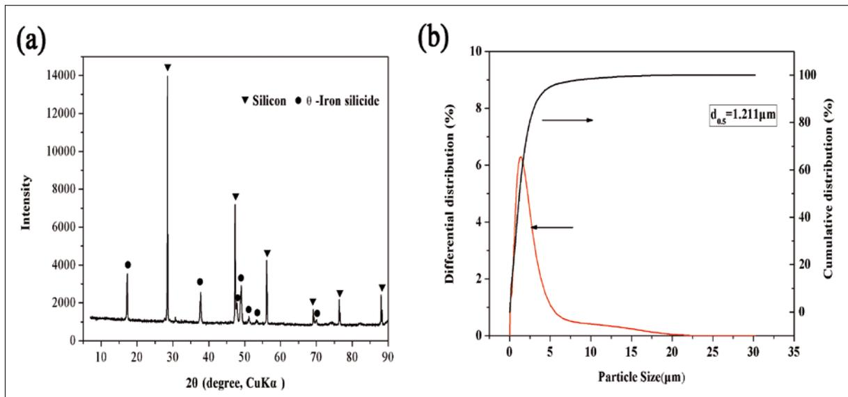
Fig. 2 a–b XRD patterns of ferrosilicon (a), and distribution of particle size of ferrosilicon (b) [22]
