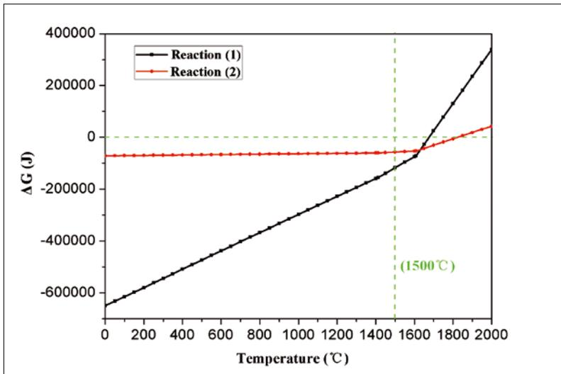
**Fig. 4** Changes in Gibbs free energy of reactions (1) and (2) as a function of temperature under 0,03 MPa N<sub>2</sub>
