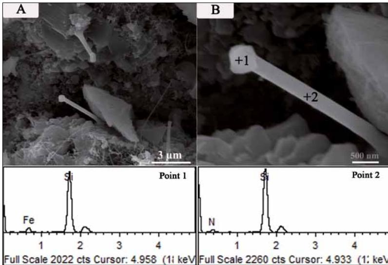
**Fig. 14** SEM micrographs of  $\text{Si}_3\text{N}_4$  whiskers with tips in sample FS-5; B: higher magnification of the  $\text{Si}_3\text{N}_4$  whiskers in A [22]
