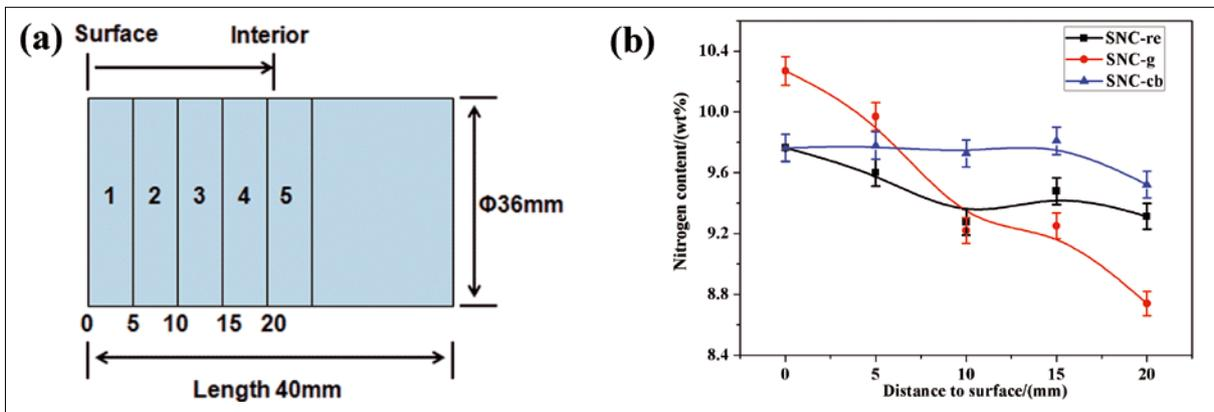
**Fig. 7 a–b** Schematic diagram of the testing wafers prepared for nitrogen content analysis (a), and the contents of nitrogen as a function of nitriding depth (from sample surface to interior) by using XRF analyser (b) [23]
