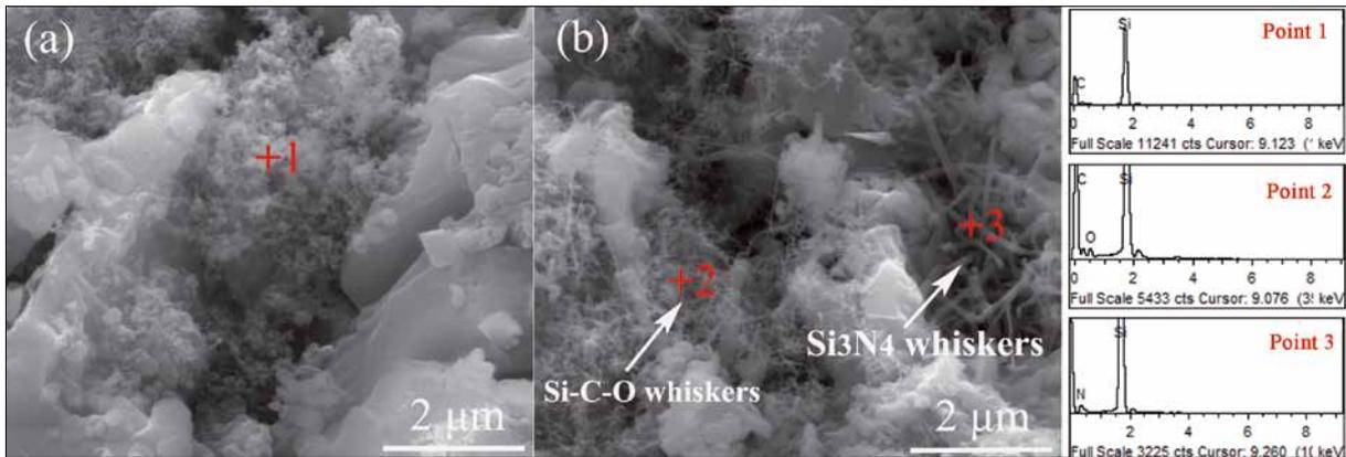
**Fig. 6 a–b** Si–C–O whiskers and nano-granules formed in sample SNC-cb matrix (SEI): a) SiC nano-granules in sample matrix, and b) Si<sub>3</sub>N<sub>4</sub> and SiC whiskers in sample interior (SEI) [23]
