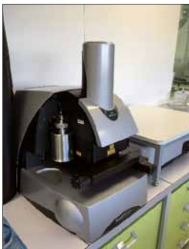
Fig. 4 Photo of the Malvern Morphologi G3SE-ID equipped with a Raman RXNN1 semiconductor laser
