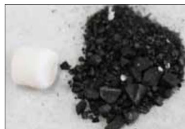
**Fig. 7** Crushed MgO pellet after the reduction test
