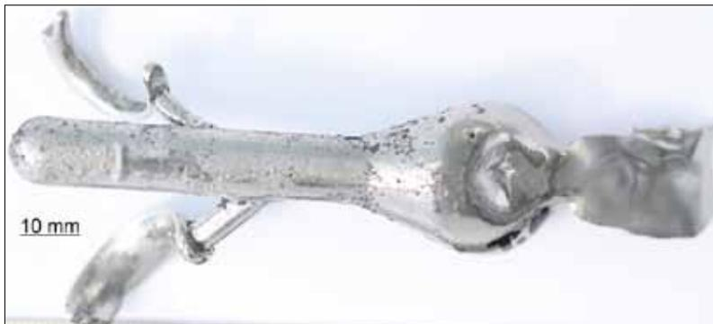
**Fig. 6** Cast part produced with investment mould with 3 coatings (the surface was smooth and shiny, suggesting that only a slight corrosion reaction occurred)
